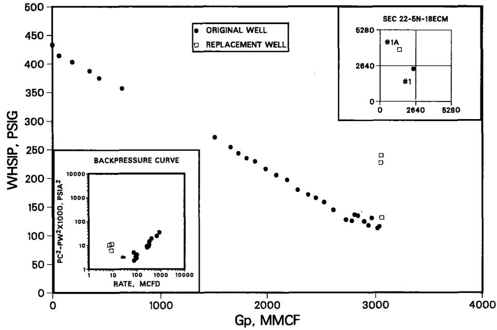
Fig. 5—RN59 pressure vs. cumulative production and backpressure plot.
