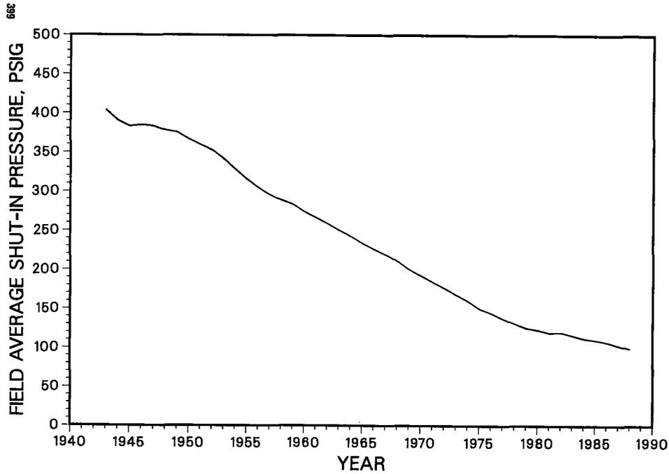
Fig. 7—Guymon-Hugoton field average shut-in pressure vs. time plot.
