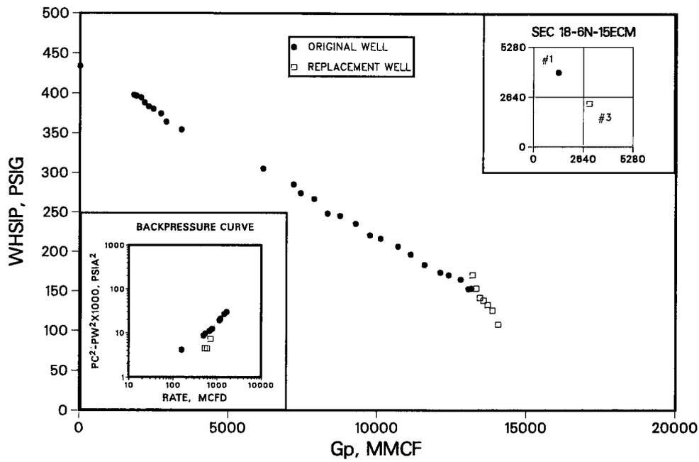
Fig. 14—RN63 pressure vs. cumulative production and backpressure plot.
