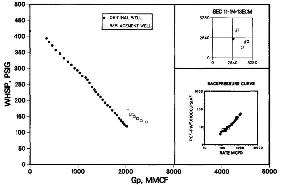
Fig. 8—RN10 pressure vs. cumulative production and backpressure plot.
