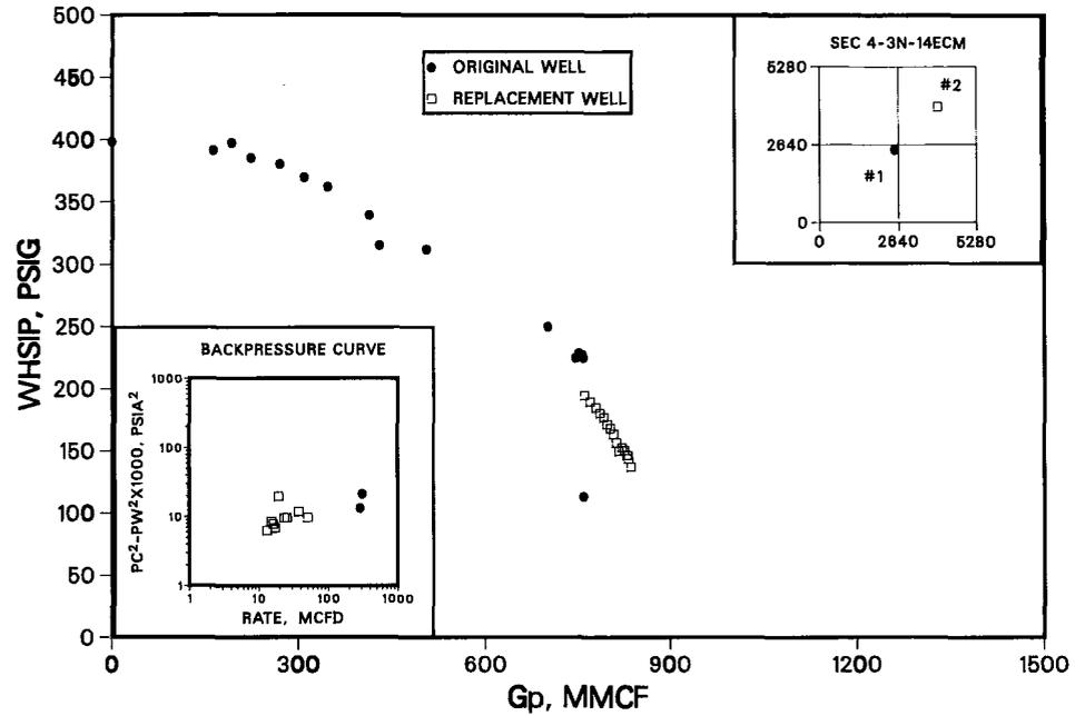
Fig. 10—RN40 pressure vs. cumulative production and backpressure plot.
