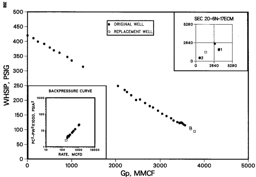
Fig. 3—RN70 pressure vs. cumulative production and backpressure plot.
