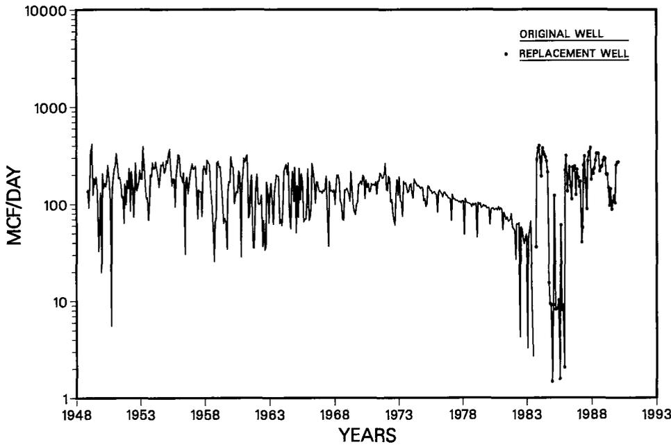
Fig. 9—RN10 production rate vs. time plot.
