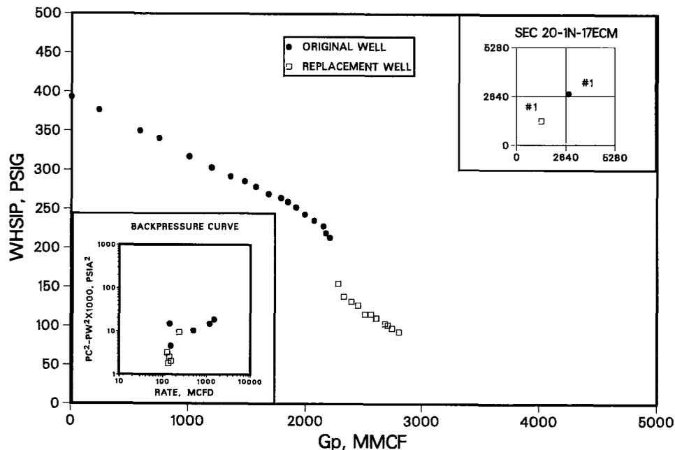
Fig. 12—RN21 pressure vs. cumulative production and backpressure plot.
