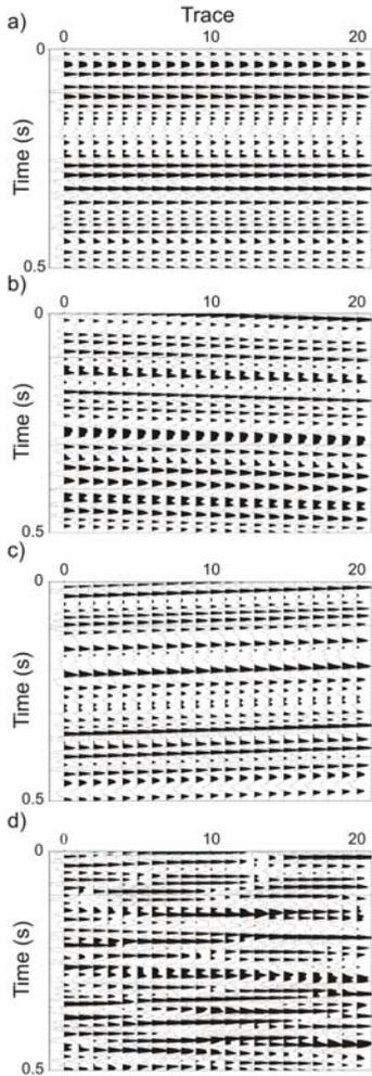
Figure 1: (a) Signal, (b) positively and (c) negatively dipping coherent noise and (d) entire data for the noise-to-signal ratio 4:1
