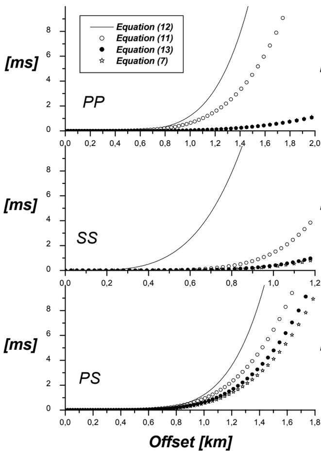
**Figure 1.** The deviation in ms from the exact traveltimes computed from model I.
