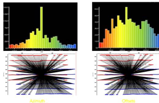
Figure 2. Analysis of azimuth and offset distribution for the original Statfjord 3D OBS survey
