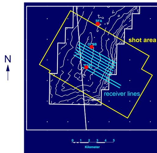
Figure 1. Acquisition Geometry for the original Statfjord 1997 3D OBS survey
