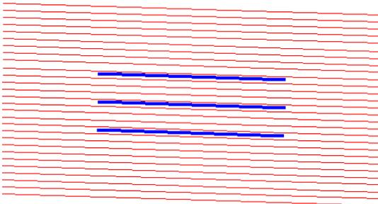
Figure 3: Acquisition geometry for Gullfaks South, with 28 source lines (red), orientated parallel to three receiver lines (blue).
