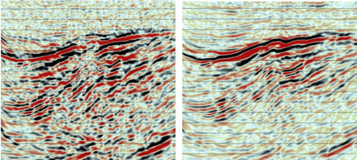
Figure 6: Improved structural resolution of 3D P-wave data (bottom), compared to 2D P-wave data (top)
