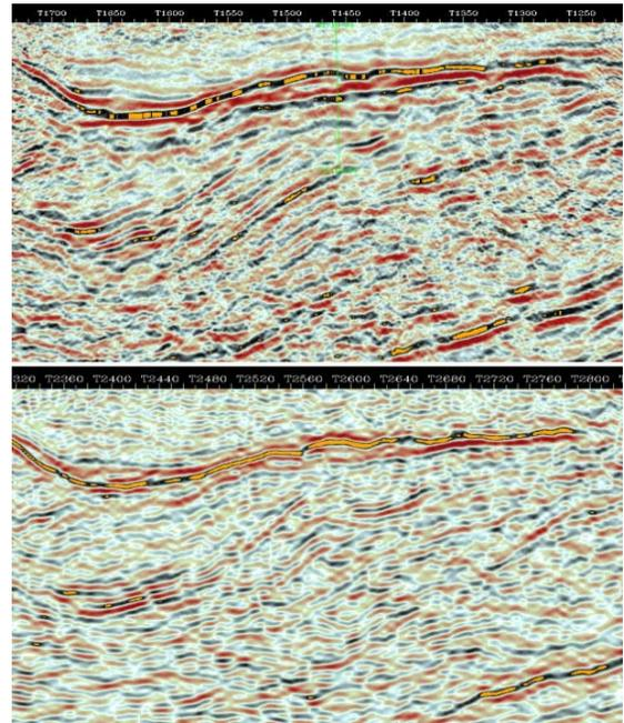
Figure 4: Enhanced structural imaging by the OBS data set (top) compared to the pre-stack depth migrated towed streamer data set (bottom). (Næss *et al.*, 2002)
