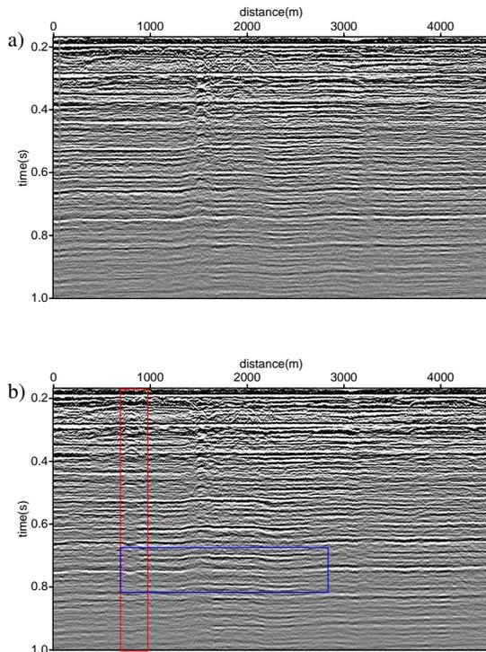
Figure 4: LOSEM data raw stack. a) 1988, b) 1990. Red box: seismic response from relief well; blue box: anomaly due to gas blow out.
