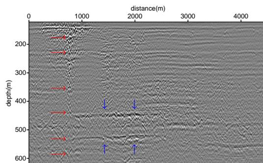
Figure 8: Time lapse diffraction image. Red arrows: relief well; blue arrows: anomaly due to gas blow out.
