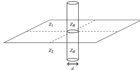
Figure 1: Parameters defining diffraction response from borehole: diameter  $d$  and impedance contrast of borehole ( $Z_B$ ) with host rock ( $Z_1, Z_2$ ).
