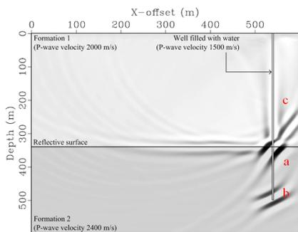
Figure 3: Seismic wave interaction with vertical well (after Lødemel, 2013).
