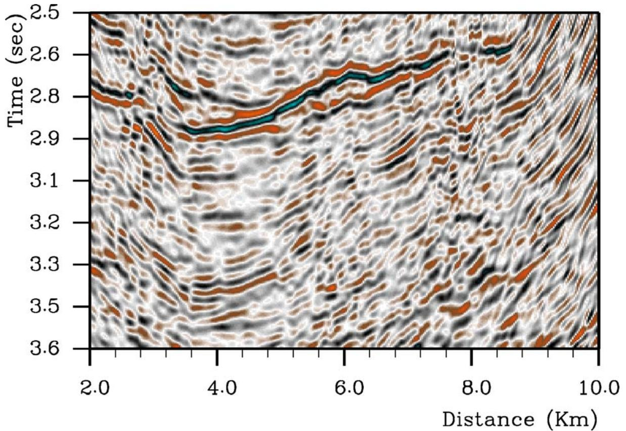
**Figure 4:** Depth migrated OBC inline 1057 using cross-line offsets up to 90 m.
