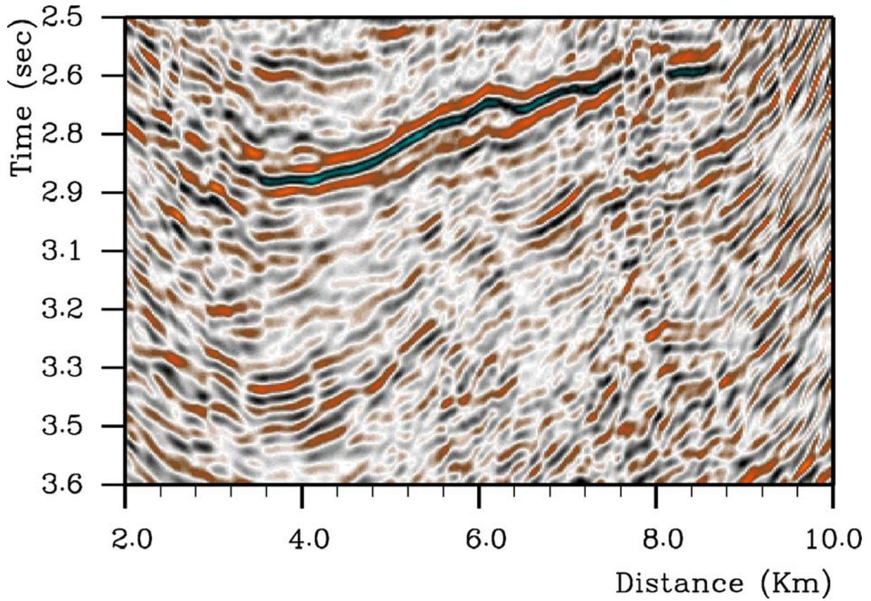
**Figure 3:** Depth migrated OBC inline 1057 using cross-line offsets up to 350 m.
