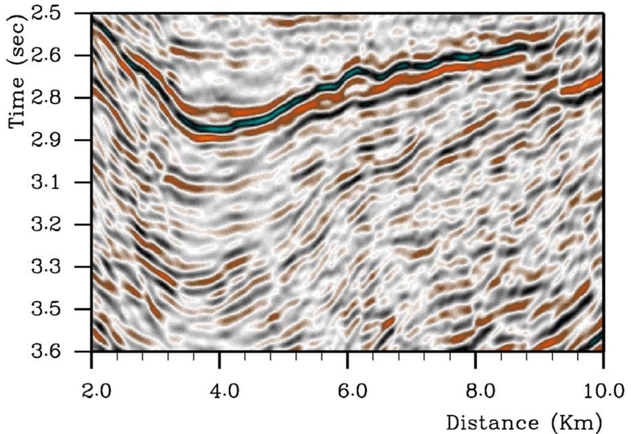
**Figure 2:** Depth migrated OBC inline 1057 using cross-line offsets up to 1.8km
