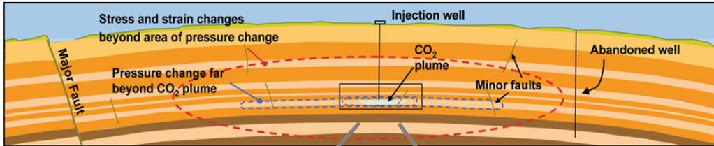
**Injection-induced stress, strain and deformation**
