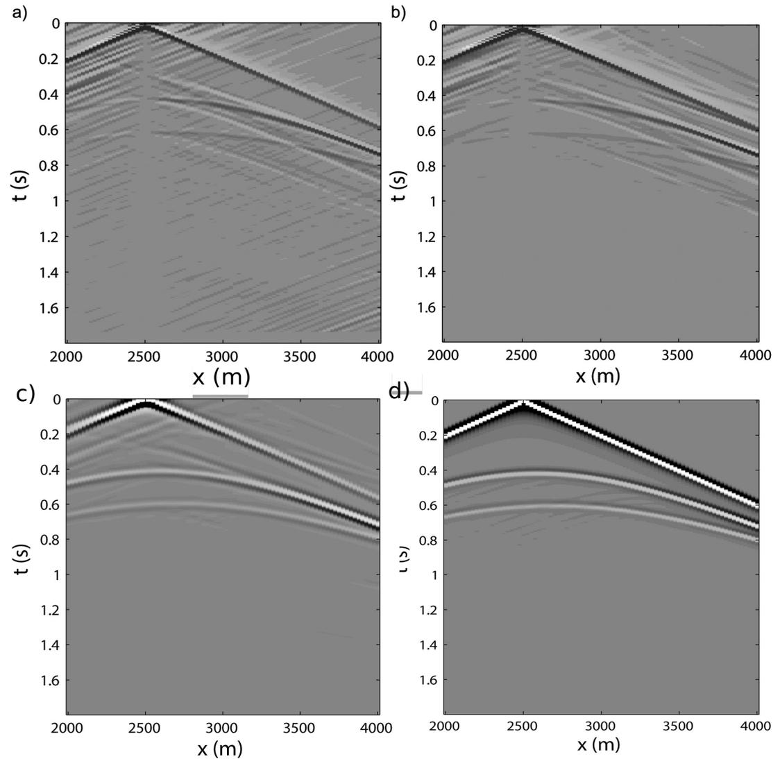
The virtual response of the source at  $x = 2500$  m retrieved by a) DC, b) CH and c) CC. d) The reference response modelled with a homogeneous overburden.
