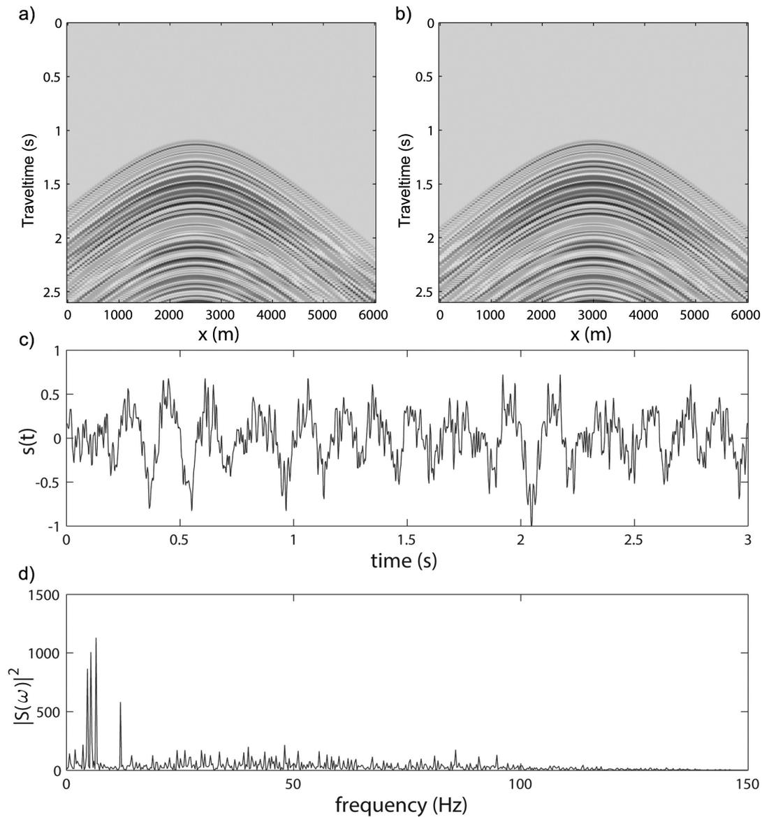
Drill-bit source function and recorded common-source gathers. a) Common-source gather at  $x = 2500$  m and b) at  $x=3000$  m. c) Modelled drill-bit source function. d) Power spectrum of the modelled drill-bit function.
