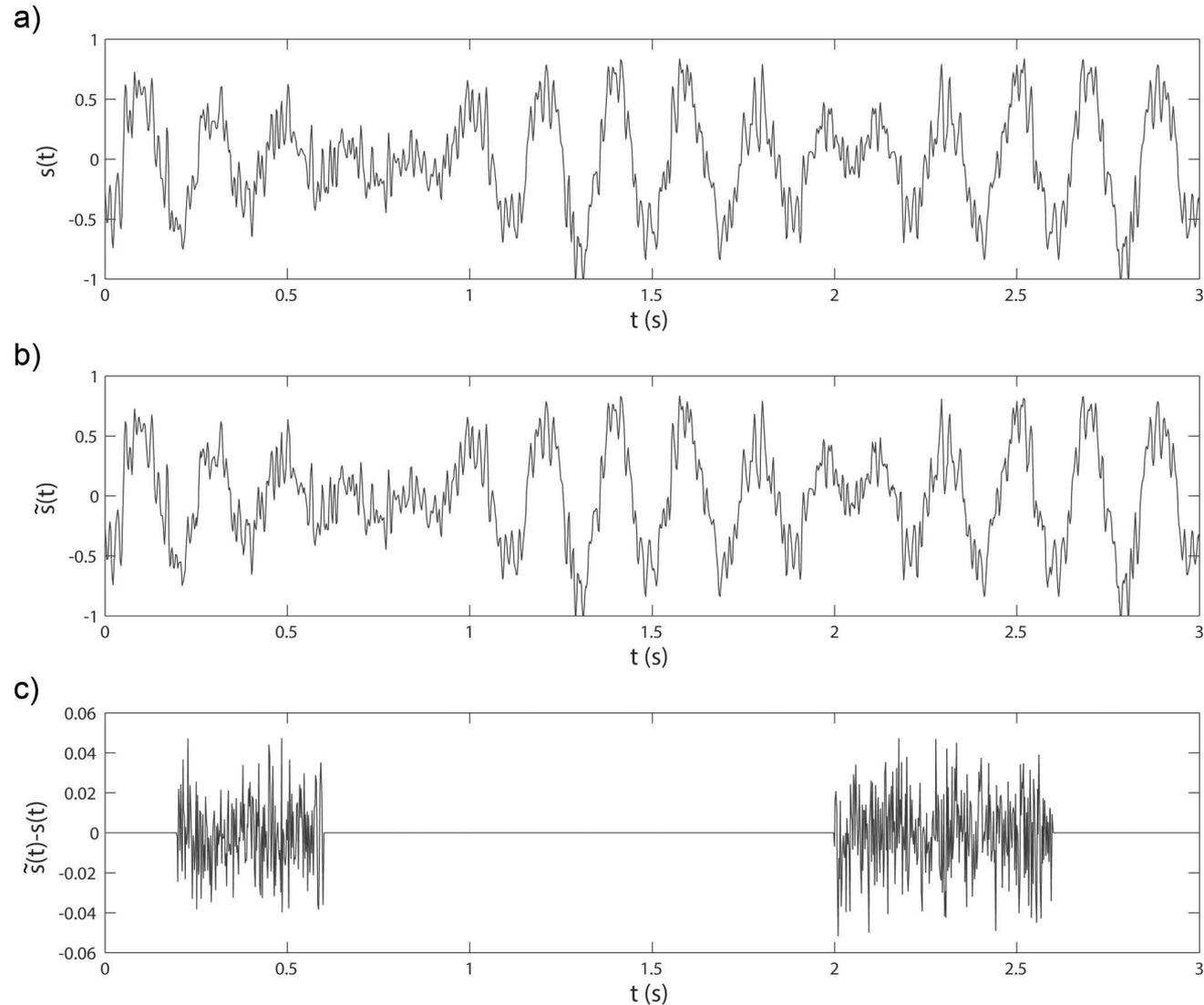
An example of the modelled drill-bit signals. a) The exact drill-bit source function  $s(t)$ . b) Estimate of the signal. c) The noise added to the estimated signal, which is up to 5% of the drill-bit signal.
