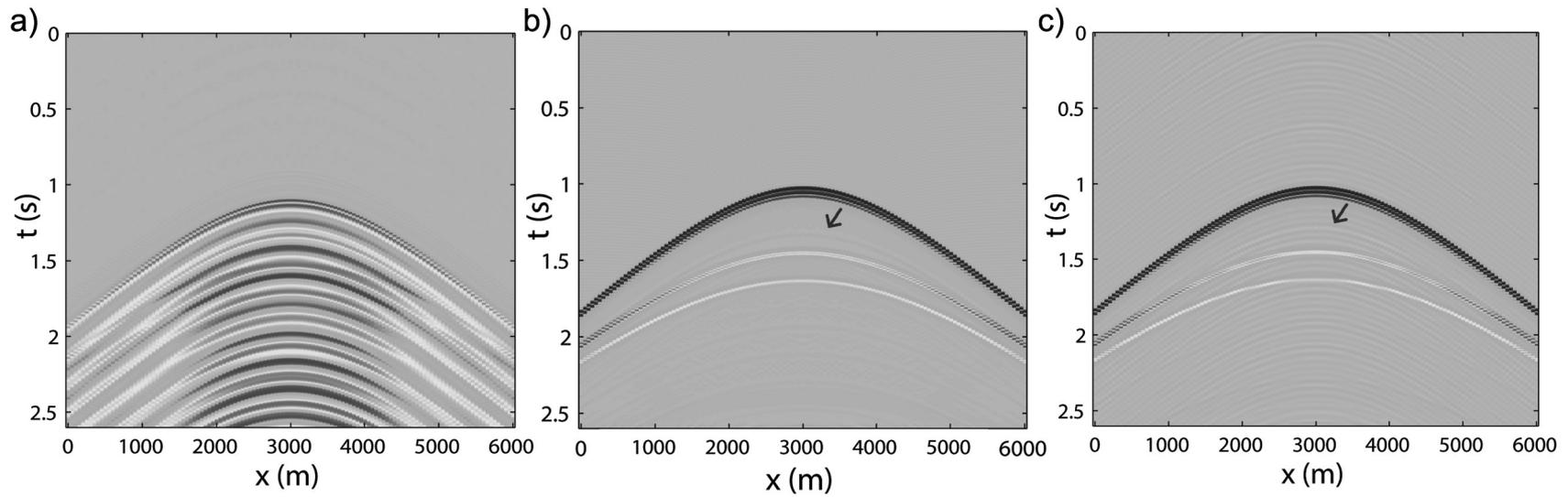
a) Raw common-source gather from drilling noise at  $x=3000$  m. Pilot-deconvolved common-source gathers using b) the exact source signal and c) the noise-contaminated pilot signal. The arrow indicates the internal multiple from the second layer, which arrives about 0.2 seconds after the direct waves.
