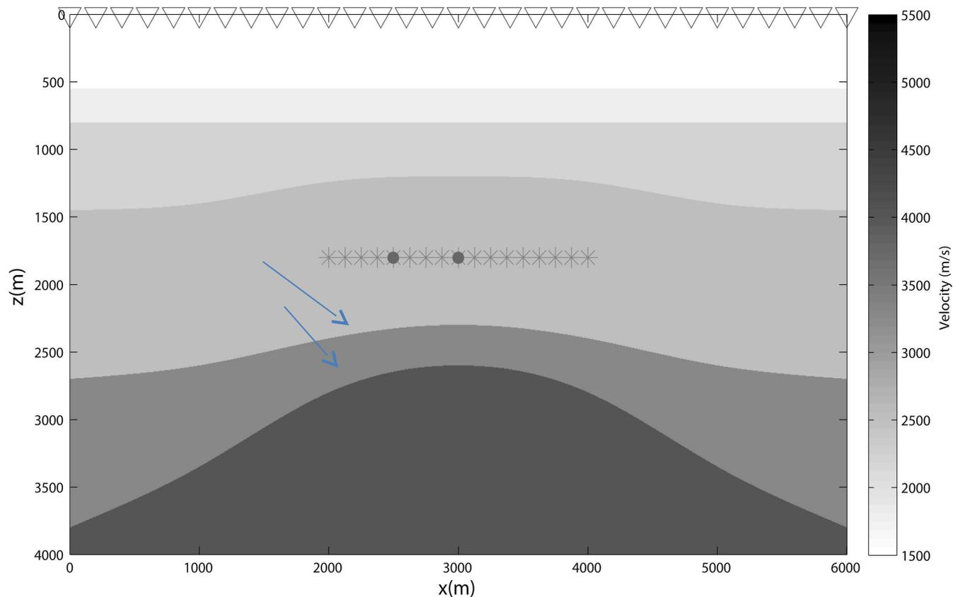
Synthetic Vp model. The stars denote drill-bit positions and triangles denote receivers at the surface level. The dots indicate two reference source positions for trace comparison.
