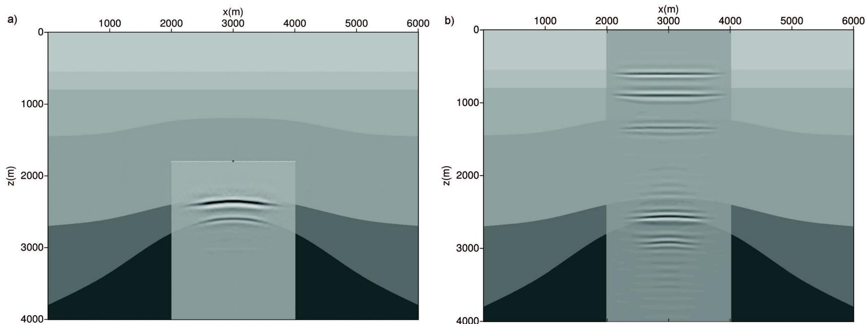
a) using retrieved virtual reflection responses at the drill-bit positions, and b) using conventional surface seismic reflection data. The background indicates the true velocity model. Image a) is obtained using a homogeneous velocity model of 2750 m/s (2500 m/s+10% error), while image b) is obtained using the 10-percent erroneous velocities of the whole model.
