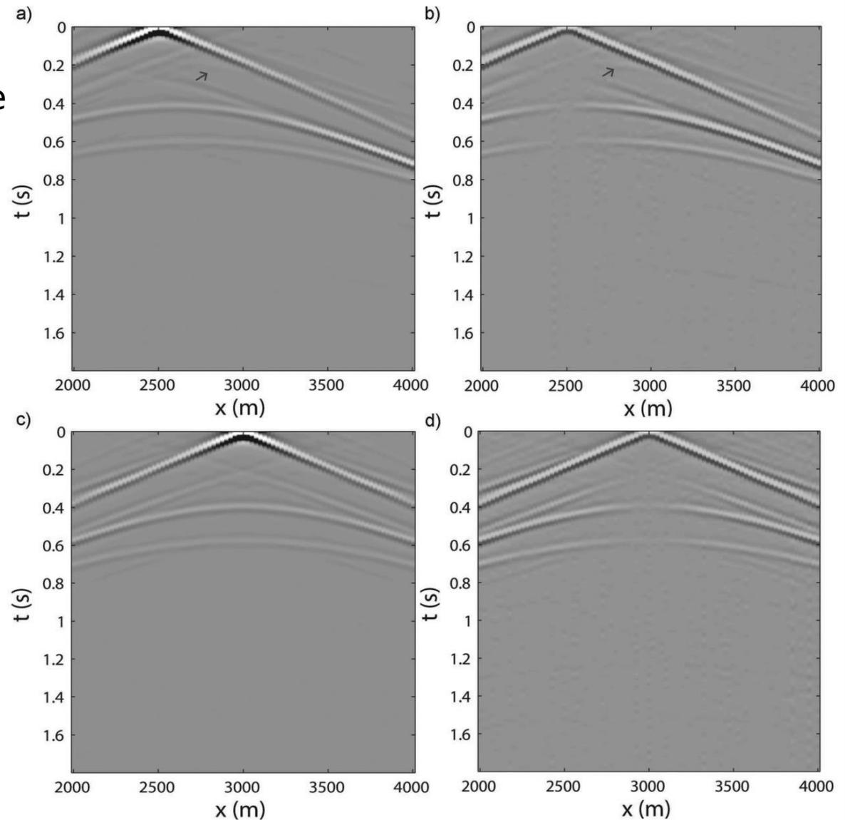
a) and c) used  $s(t)$  for pilot deconvolution. b) and d) use  $\tilde{s}(t)$ , and energy normalization is applied afterwards. The arrow indicates the non-physical reflection identified as the crosscorrelation of the direct waves and the internal multiples.
