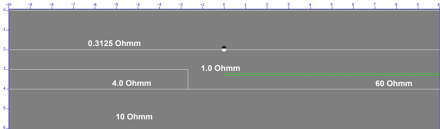
Resistivity/conductivity model maps into velocity model
