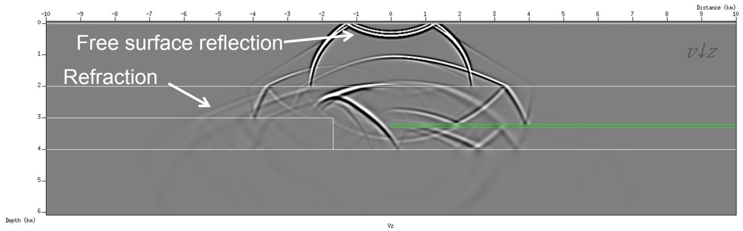
Air-water reflection at seabed after  $\sim 2.7$  s (4000 m / 1500 m/s)
