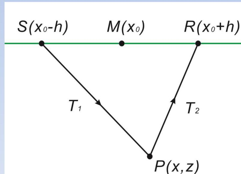
**Figure 1** Schematic plot of scattering ray propagating in homogeneous TTI media
