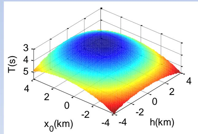
**Figure 3** Traveltime as a function of half offset  $h$  and midpoint  $x_0$  for isotropic case (top left), VTI case with  $\eta = 0.2, \delta = 0.1$  (top right), tilted elliptical isotropic (TEI) medium with  $\eta = 0, \delta = 0.1$  and  $\theta = 30^\circ$  (bottom left) and TTI case with  $\eta = 0.2, \delta = 0.1$  and  $\theta = 30^\circ$  (bottom right). On-axis velocity is 2 km/s. The two-way zero-offset traveltime is 3 s.
