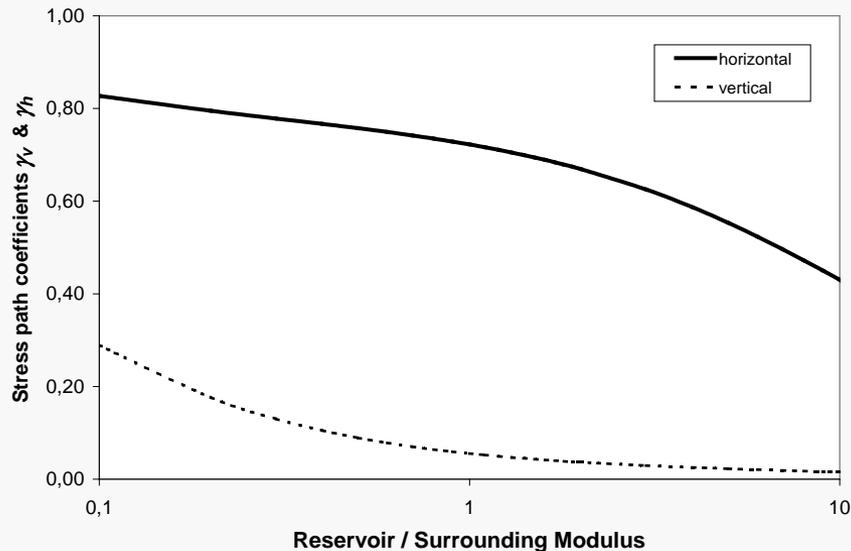
Effect of elastic (shear modulus) mismatch:
