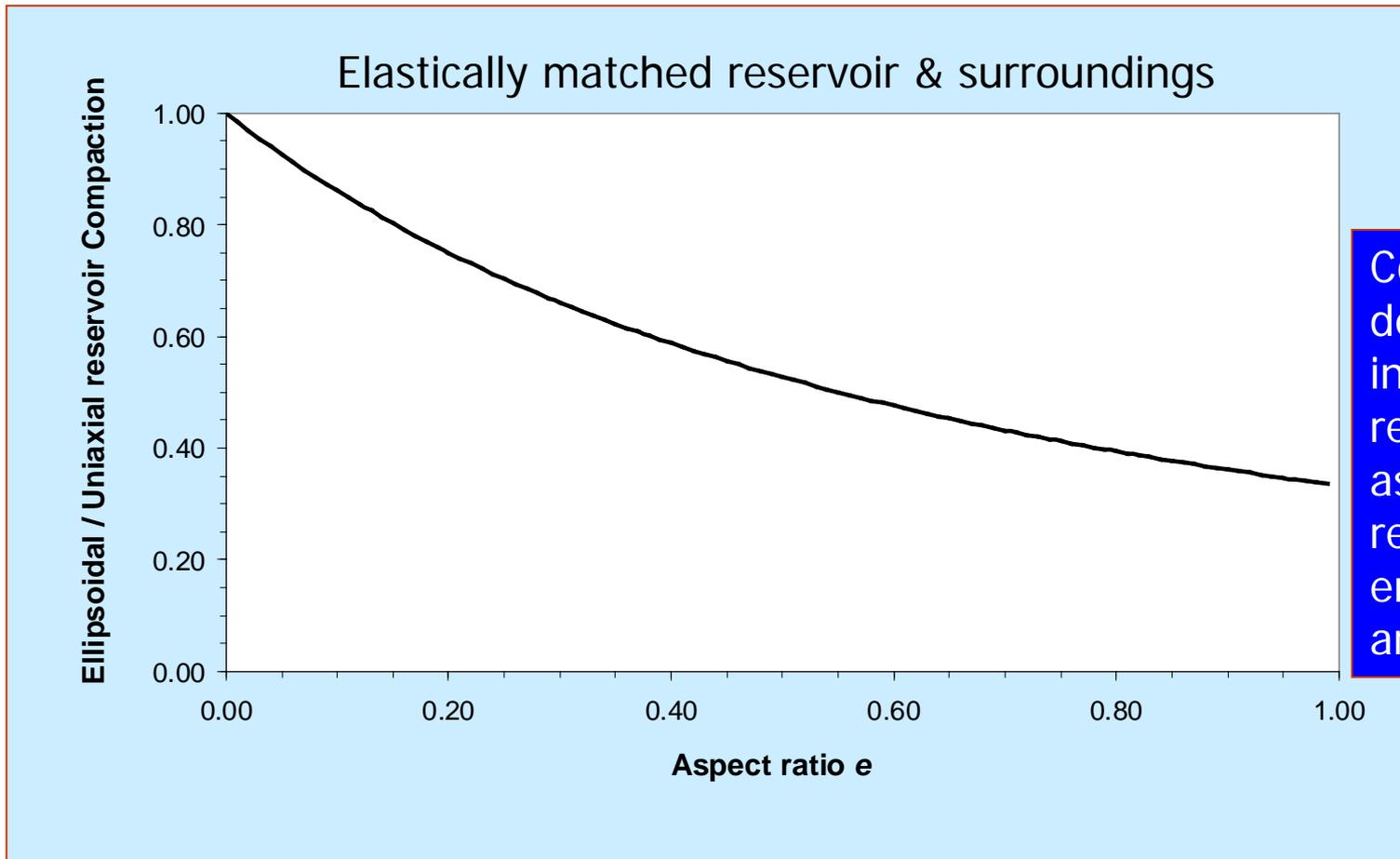
Compaction decreases with increasing reservoir aspect ratio, reflecting enhanced arching
