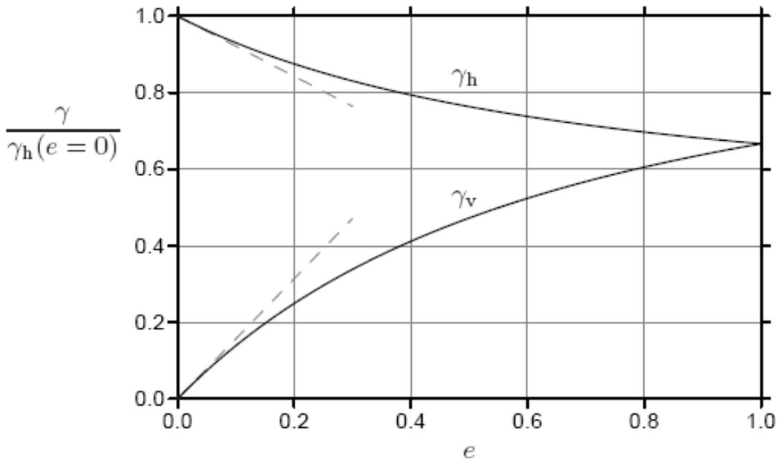
Only for [European] pancake shaped reservoir ( $e=0$ ) is the uniaxial strain & no arching assumption fulfilled.
