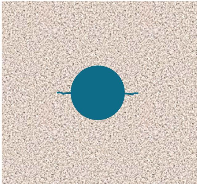
The leak-off point is controlled by the stress state at the borehole wall, which differ from the in situ stress state.
