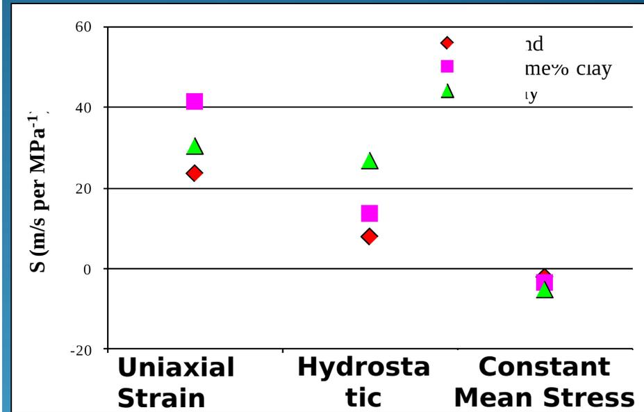
Stress sensitivity of axial P-wave velocity for 3 different stress paths
