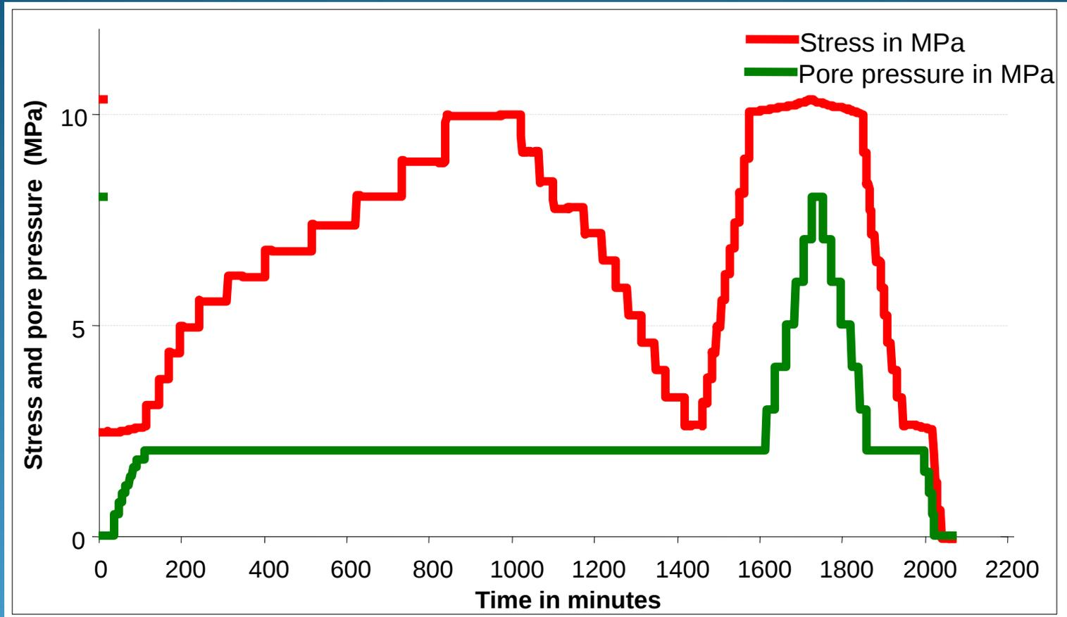
Example taken from test of sample with high clay content
