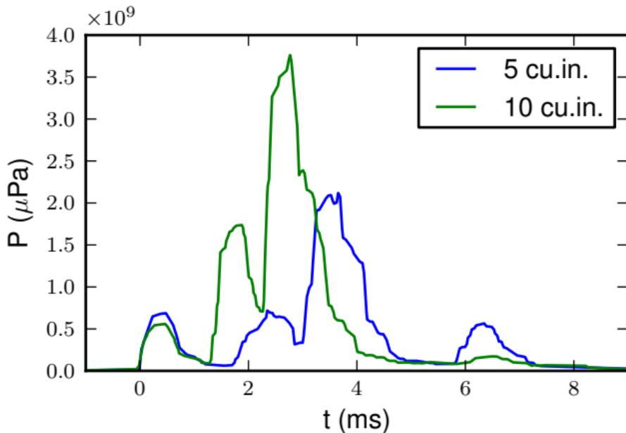
Figure: RMS values of signal, calculated with a window width of 0.5 ms
