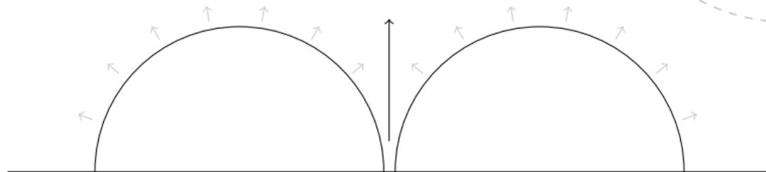
**Figure:** High-velocity flow created by the merging of separate bubbles
