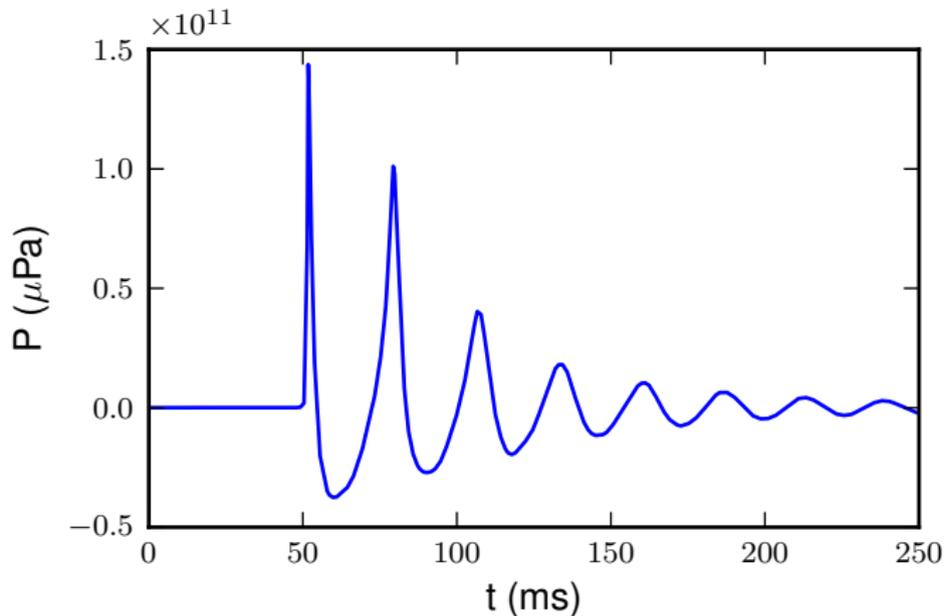
Figure: 10 cu.in. shot, hydrophone 2 (normalised to 1 m)
