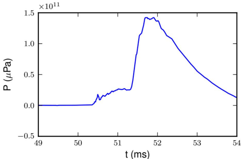
Figure: 10 cu.in. shot, hydrophone 2 (normalised to 1 m)
