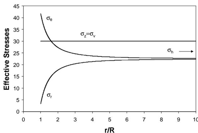
Figure 2: Stress state near a vertical borehole, showing the splitting of the horizontal far field stress into a radial and a tangential principal stress component near the borehole wall ( $r$ : distance from wall;  $R$ : borehole radius). From Fjær & Holt (1999).
