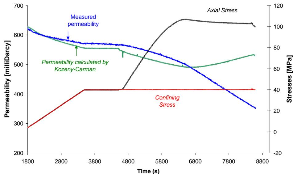
Figure 7: Permeability measured during a triaxial test with Red Wildmoor sandstone. Also shown is the permeability as predicted by the Kozeny-Carman equation, using only the porosity term, derived from bulk strain measurements on the core. From Lutnes (1999).
