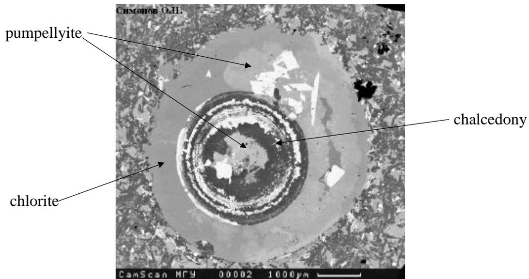
Figure 6. The amygdale in plateau basalt from Siberian platform (Russia). Scanning image.
