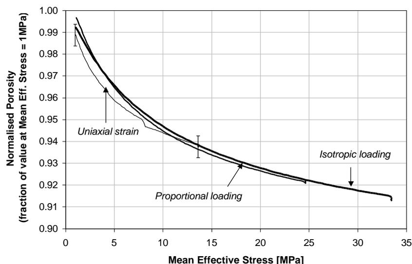
Figure 6: Porosity correction factor vs. mean effective stress for the 3 different stress paths employed. Porosity values are normalised with respect to measurements at 1.5 MPa confining and 0.5 MPa pore pressure. From Holt et al. (2001).
