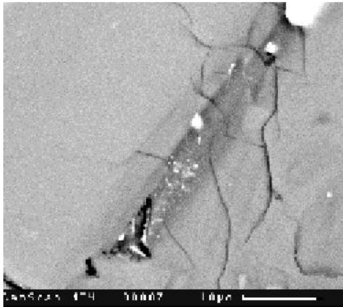
Figure 5. Microfractures in modern basalt from Kluchevskoy volcano (Kamchatka). Scanning image.
