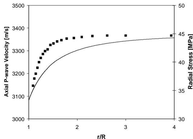
Figure 3: P-wave velocity vs distance from borehole wall, based on laboratory tests with synthetic sandstone undergoing a stress path similar to that of a rock near a borehole (cf Figure 2). From Fjær & Holt (1999).
