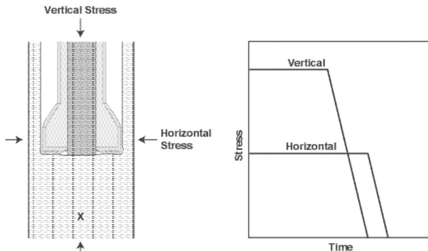
Figure 4: Sketch of stress release occurring during coring in a vertical well. From Holt *et al.* (2000).
