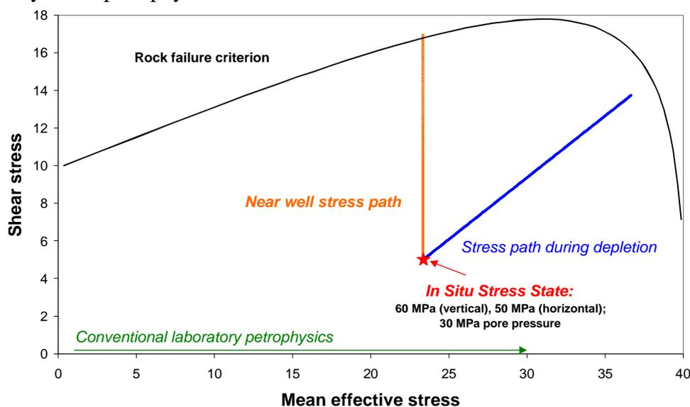
Figure 1: Illustration of states of stress occurring in a reservoir during depletion, in the vicinity of a borehole during logging, and in the laboratory during most types of conventional petrophysical measurements.
