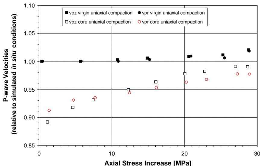
Figure 5: P-wave velocities of virgin and simulated core synthetic sandstones, showing the larger stress sensitivity of the cores. From Holt (1999).
