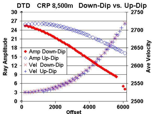
Figure 4: Amplitudes and average velocities for raypaths in CRP centered at 8500 meters along the dipping salt model.
