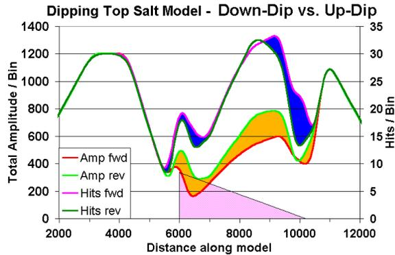
**Figure 5:** Comparison of CMP amplitude and fold along the model. The differences between the up-dip and down-dip results are color filled. The pink triangle shows the lateral position and shape of the salt body.
