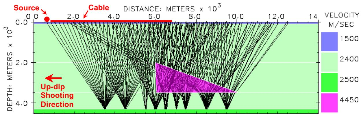
**Figure 1:** Computer model of simple salt shape with flat bottom and dip on top of salt of 20 degrees. Black lines are raypaths to selected common-reflection-point gathers from the right to left shoot (termed "up-dip" in this paper). For clarity only every fourth ray is plotted. The position of the hydrophone cable is shown for the shot at 600 meters along the model.
