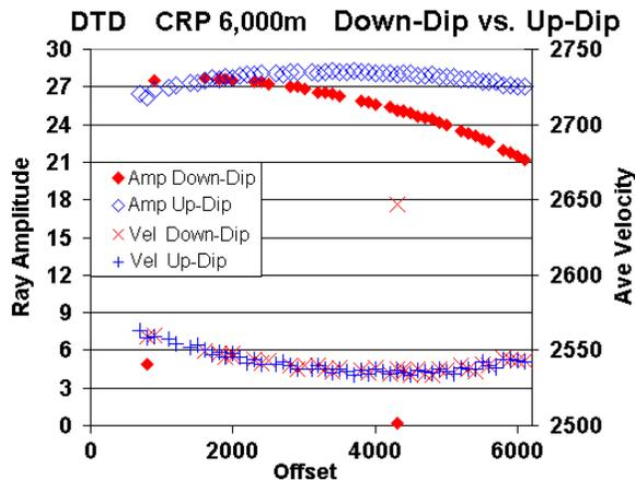
Figure 3: Amplitudes and average velocities for raypaths in CRP centered at 6000 meters along the dipping salt model. The amplitudes for the line shot left to right (down-dip) are marked as red diamonds, the up-dip line in blue. Note the amplitudes diverge as offset increases.
