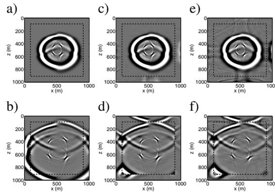
**Figure 1** Vertical profiles of snapshots of vertical particle velocity at two different times (0.2 and 0.3 s). Figures a) and b) are exact reproductions; c) and d) are reconstructed with Dirichlet boundary method; e) and f) are reconstructed with the Kirchhoff integral method. The black stippled lines mark the boundaries where the fields are stored, and inside which the wavefields are reverse-time reconstructed.
