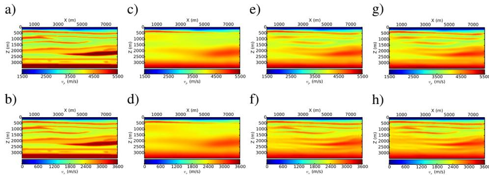
**Figure 2** Vertical profiles of a) true  $V_p$ ; b) true  $V_s$ ; c) initial  $V_p$ ; d) initial  $V_s$ ; e) inverted  $V_p$  using Dirichlet boundary method; f) inverted  $V_s$  using Dirichlet boundary method; g) inverted  $V_p$  using Kirchhoff integral method; h) inverted  $V_s$  using Kirchhoff integral method.
