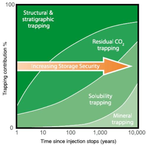
Figure 1 Various mechanisms for trapping of CO<sub>2</sub>. From [1].
