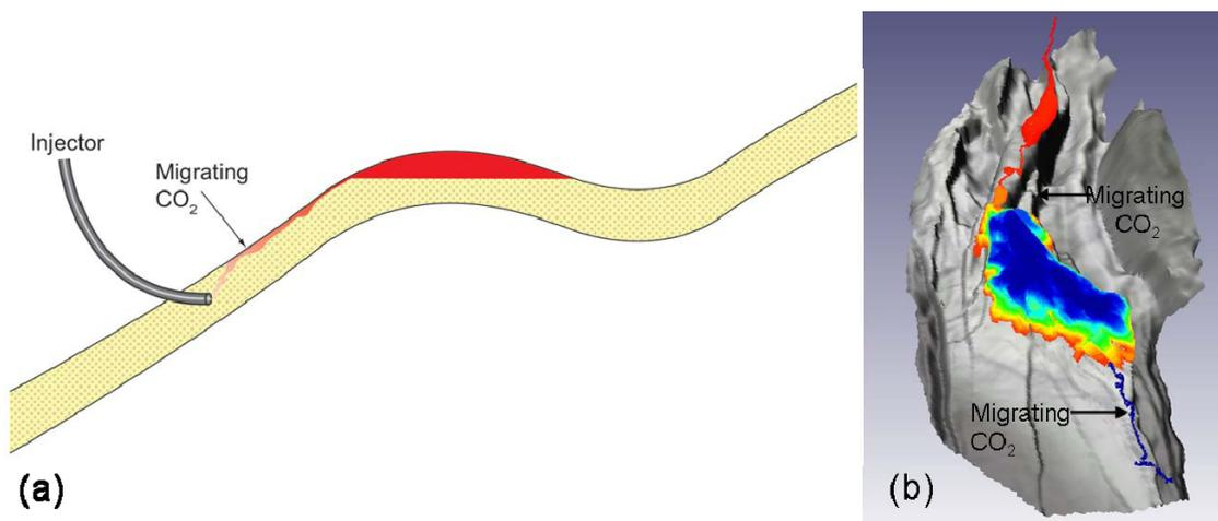
Figure 2 (a) Cross-section and (b) map view of CO<sub>2</sub> that migrates and saturates parts of a rock volume.
