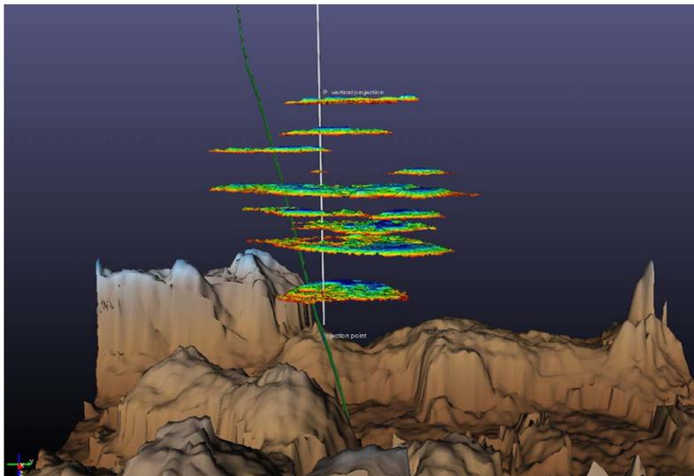
Figure 8 Distribution of bright amplitudes, converted to CO<sub>2</sub> column heights, in the nine CO<sub>2</sub>-saturated layers of the Utsira Formation. A flat CO<sub>2</sub>-water contact was applied for the construction of this figure. Courtesy of Permedia Inc.
