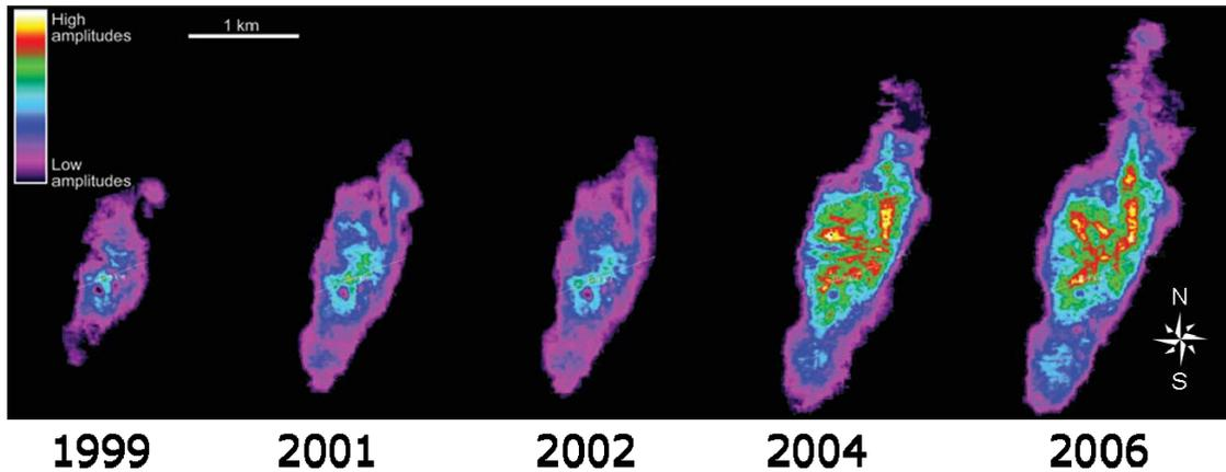
Figure 7 Accumulated total reflection amplitude from all nine layers of the Sleipner CO<sub>2</sub> plume.
