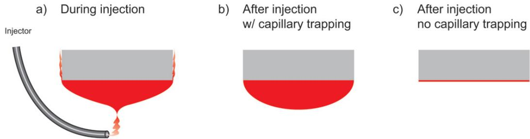
Figure 4 Capillary trapping. (a) CO<sub>2</sub> injection below an impermeable seal. (b) CO<sub>2</sub> distribution after injection with capillary trapping. (c) CO<sub>2</sub> distribution after injection, no capillary trapping. The seal is in grey and the CO<sub>2</sub> is in red.
