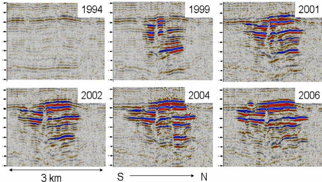
Figure 6 Time lapse seismic data in the Utsira Formation. The bright amplitudes reveal the presence of injected CO<sub>2</sub>.
