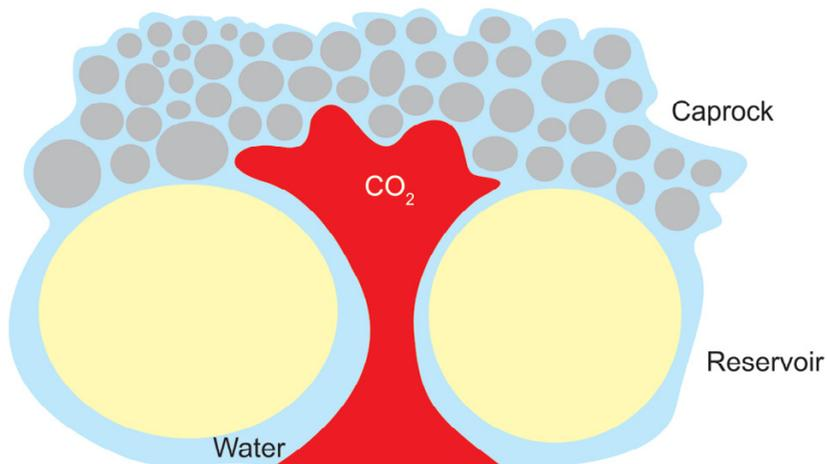
Figure 3 Capillary trapping at pore scale. Breakthrough occurs when the buoyancy results in radius  $r$  in the  $\text{CO}_2$  stringer that is small enough to allow the  $\text{CO}_2$  to invade the caprock pores.
