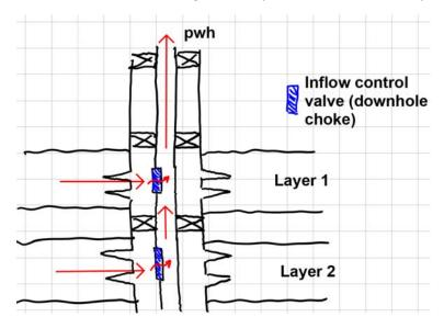
**Task 1. (10 points)** If one desires to produce a total rate from the well of 150 000 Sm3/d, split in layer 1: 50 000 Sm3/d and from layer 2: 100 000 Sm3/d, at a wellhead pressure of 10 bara, **calculate the deltap** across the inflow control valves of each layer to achieve this.
