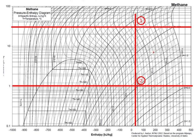
The outlet of the choke has the same enthalpy than point 1, and we have the pressure, therefore we can locate the outlet point (2)
