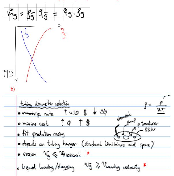
The profile of local gas rate versus depth is useful e.g. to calculate the local gas velocity and evaluate if there will be risk of erosion or liquid loading in any tubing location.
