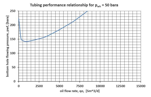
**Task 1.** Is is possible for the well to produce 4000 Sm3/d by natural flow? If not, estimate the pressure boost required by the ESP pump located downhole.
