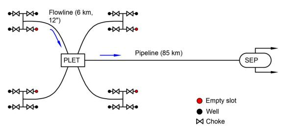
All wells are identical (in layout, productivity and all other design and operation parameters) and produce from the same reservoir. You can also assume that a simple gas material balance is good enough to represent its behavior.
