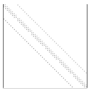
Coefficient matrix for cylindrical system. Key difference from rectangular system are the connections between blocks where j=1 with blocks where j=8
