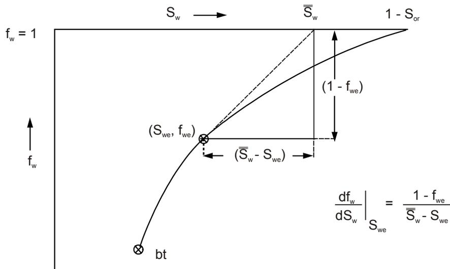
**Fig. 10.15 Application of the Welge graphical technique to determine the oil recovery after water breakthrough**
