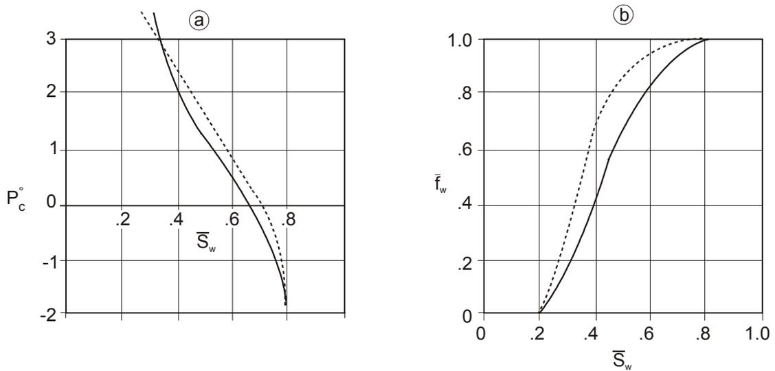
Fig. 10.39 (a) Pseudo capillary pressure, and (b) fractional flow curves for the three layered reservoir, fig. 10.34). (—high permeability at top; - - -at base of the reservoir).
