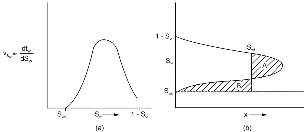
**Fig. 10.11 (a) Saturation derivative of a typical fractional flow curve and (b) resulting water saturation distribution in the displacement path**
