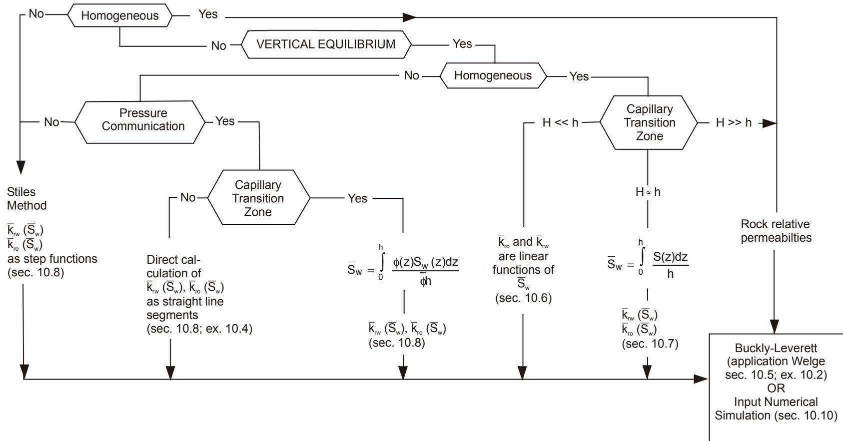
**Fig. 10.43** Methods of generating averaged relative permeabilities, as functions of the thickness averaged water saturation, dependent on the homogeneity of the reservoir and the magnitude of capillary transition zone (H). The chart is only applicable when the vertical equilibrium condition pertains or when there is a total lack of vertical equilibrium
