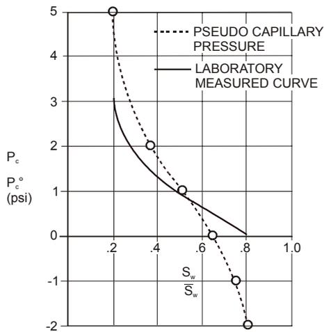
**Fig. 10.31** Capillary and pseudo capillary pressure curves.
