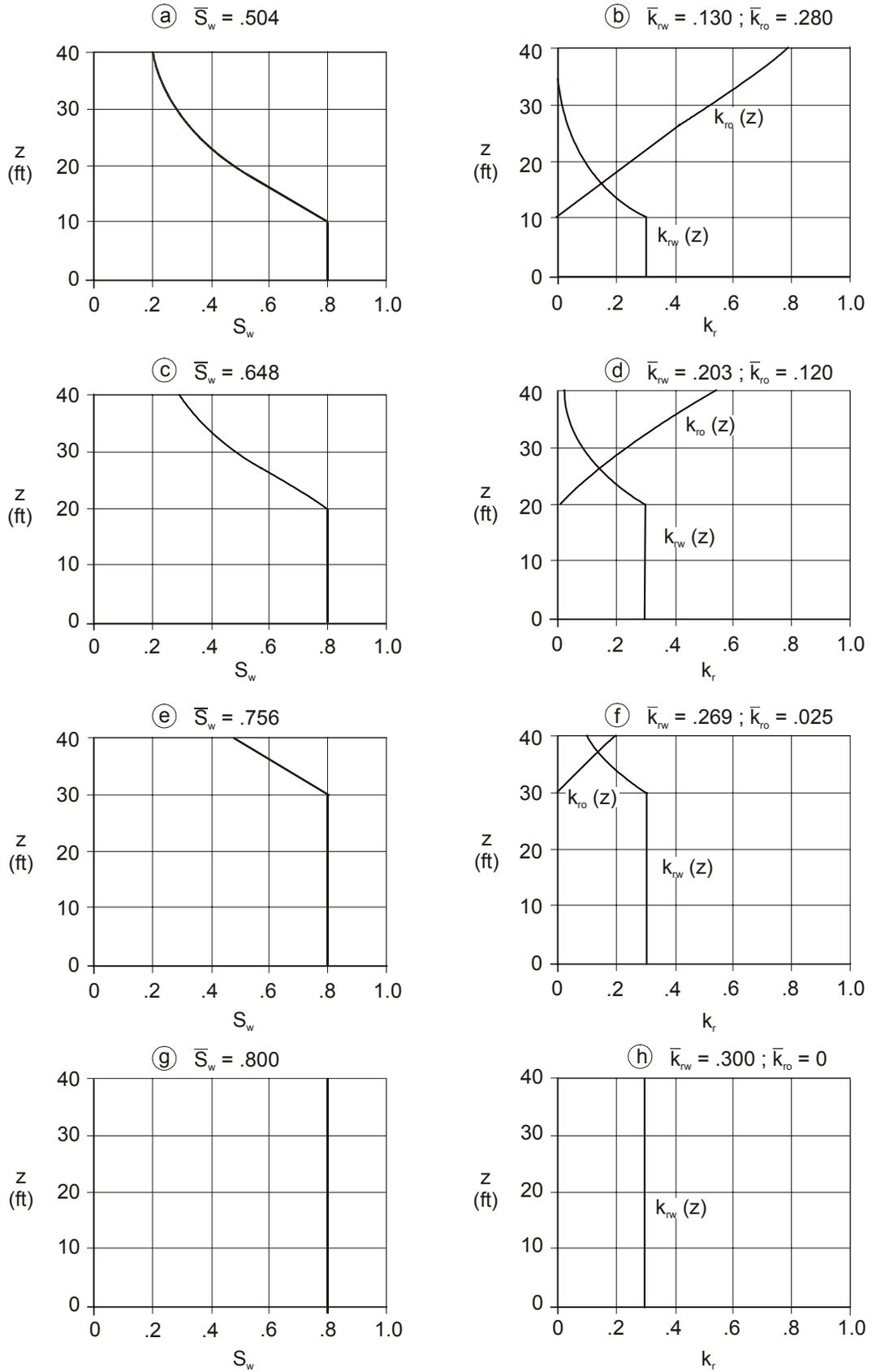
**Fig. 10.29** Water saturation and relative permeability distributions, as functions of thickness, as the maximum saturation,  $S_w = 1 - S_{or}$ , is allowed to rise in 10 foot increments in the reservoir
