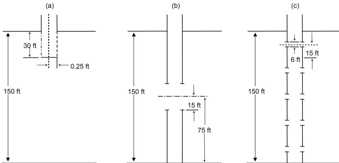
**Fig. 7.31** Examples of partial well completion showing; (a) well only partially penetrating the formation; (b) well producing from only the central portion of the formation; (c) well with 5 intervals open to production (After Brons and Marting<sup>19</sup>)
