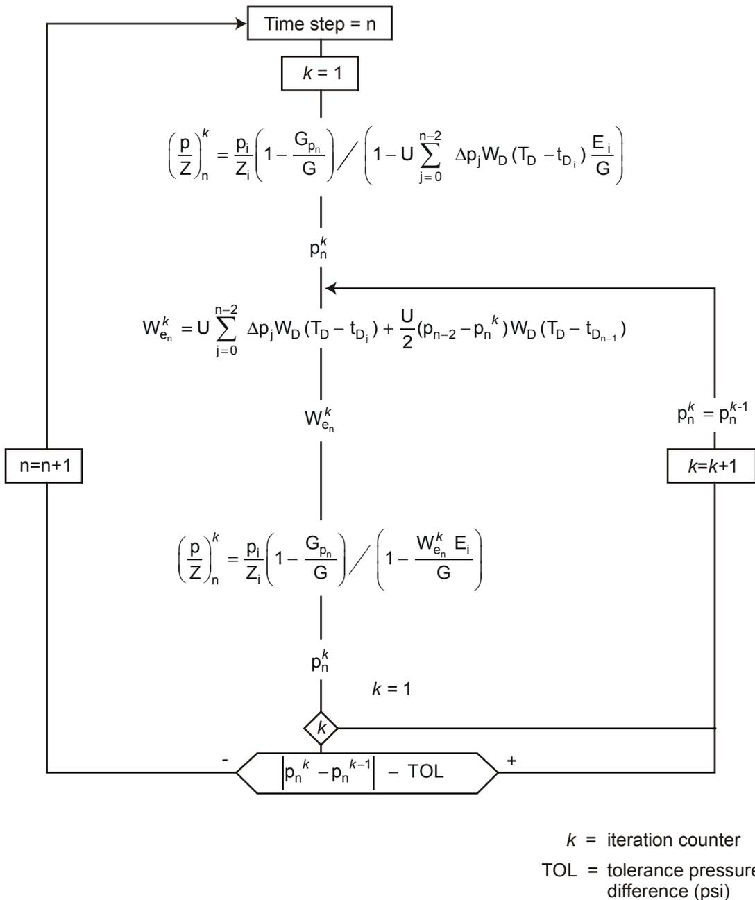
**Fig. 9.19 Prediction of gas reservoir pressures resulting from fluid withdrawal and water influx (Hurst and van Everdingen)**
