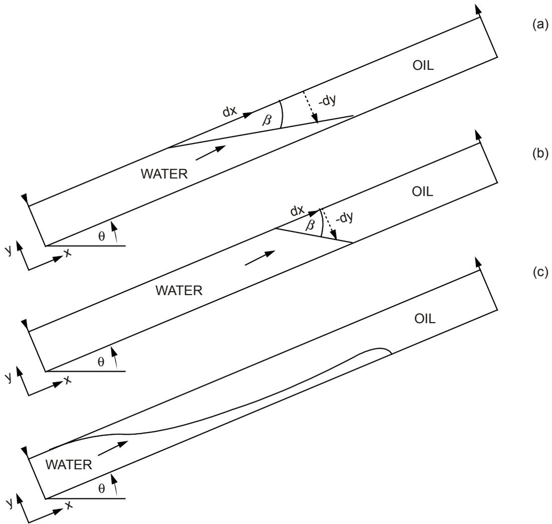
**Fig. 10.19** Illustrating the difference between stable and unstable displacement, under segregated flow conditions, in a dipping reservoir; (a) stable:  $G > M-1$ ;  $M > 1$ ;  $\beta < \theta$ . (b) stable:  $G > M-1$ ;  $M < 1$ ;  $\beta > \theta$ . (c) unstable:  $G < M-1$ .
