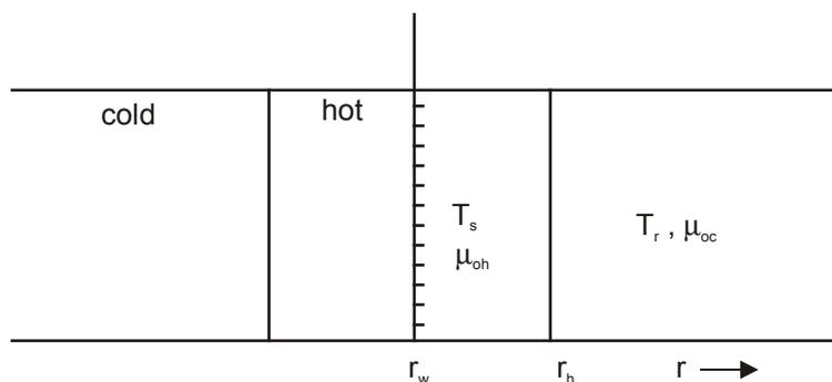
**Fig. 9.21** Conditions prior to production in a steam soak cycle
