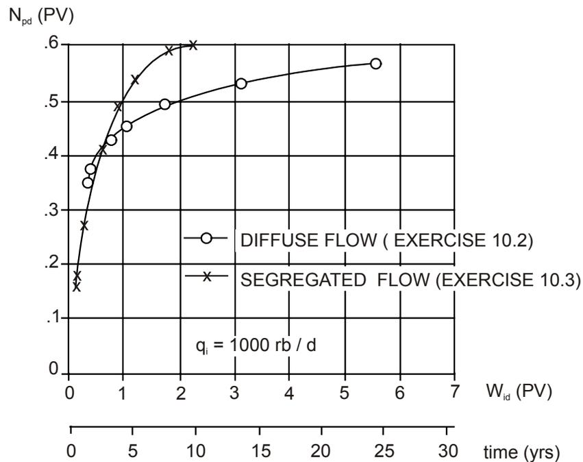
Fig. 10.24 Comparison of the oil recoveries obtained in exercises 10.2 and 10.3 for assumed diffuse and segregated flow, respectively
