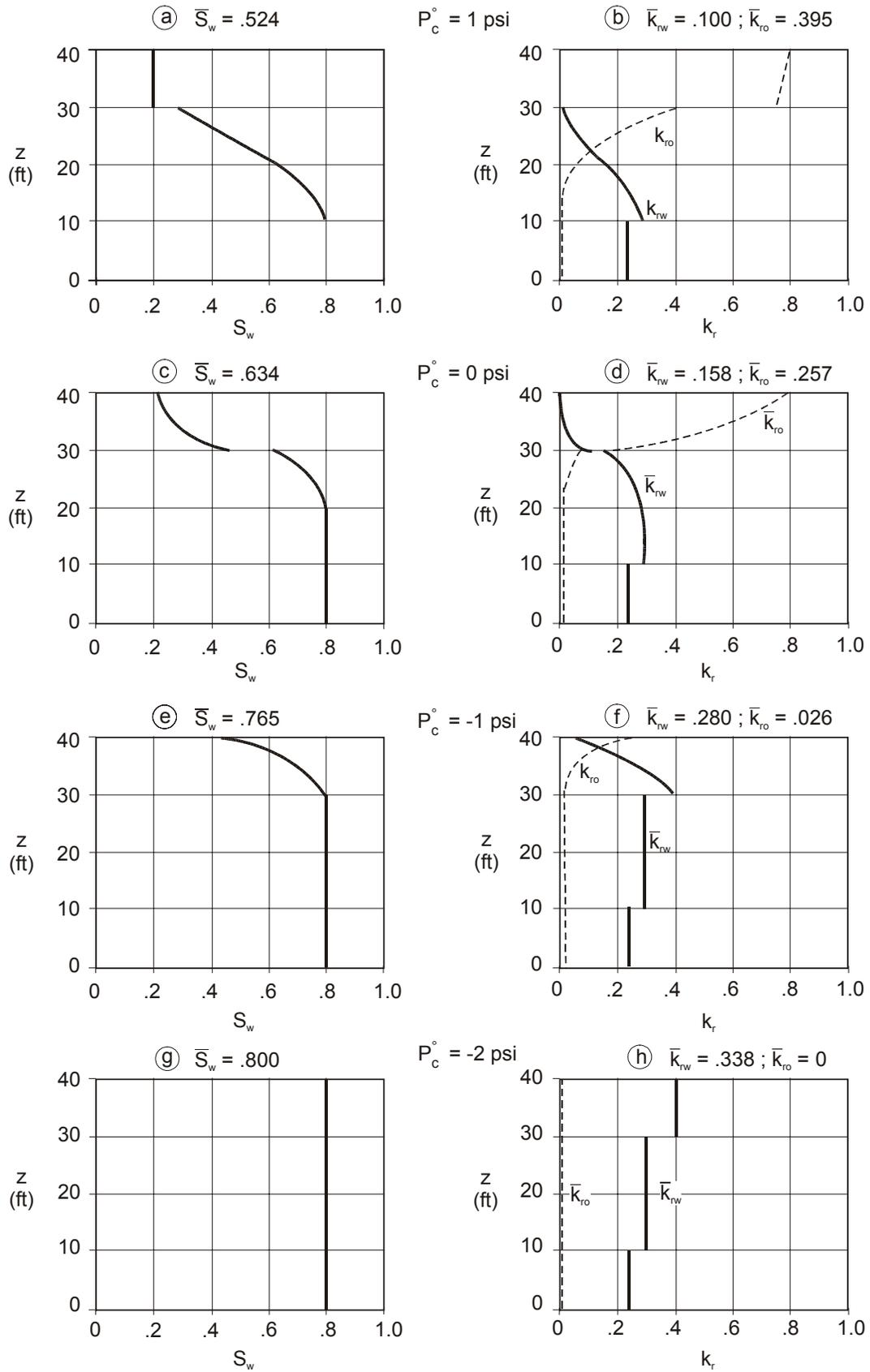
Fig. 10.37 (a)-(h) Water saturation and relative permeability distributions, as functions of thickness, for various selected values of  $P_c^\circ$  (three layered reservoir, fig 10.34)
