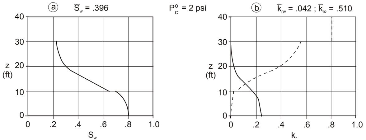
**Fig. 10.36 (a) Water saturation, and (b) relative permeability distributions, with respect to thickness, when the saturation at the base of the layered reservoir (fig. 10.34) is  $S_w = 1 - S_{or}$  ( $P_c^o = 2$  psi)**
