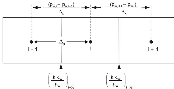
Fig. 10.45 Spatial linkage of the finite difference formulation of the left hand side of equ (10.83).
