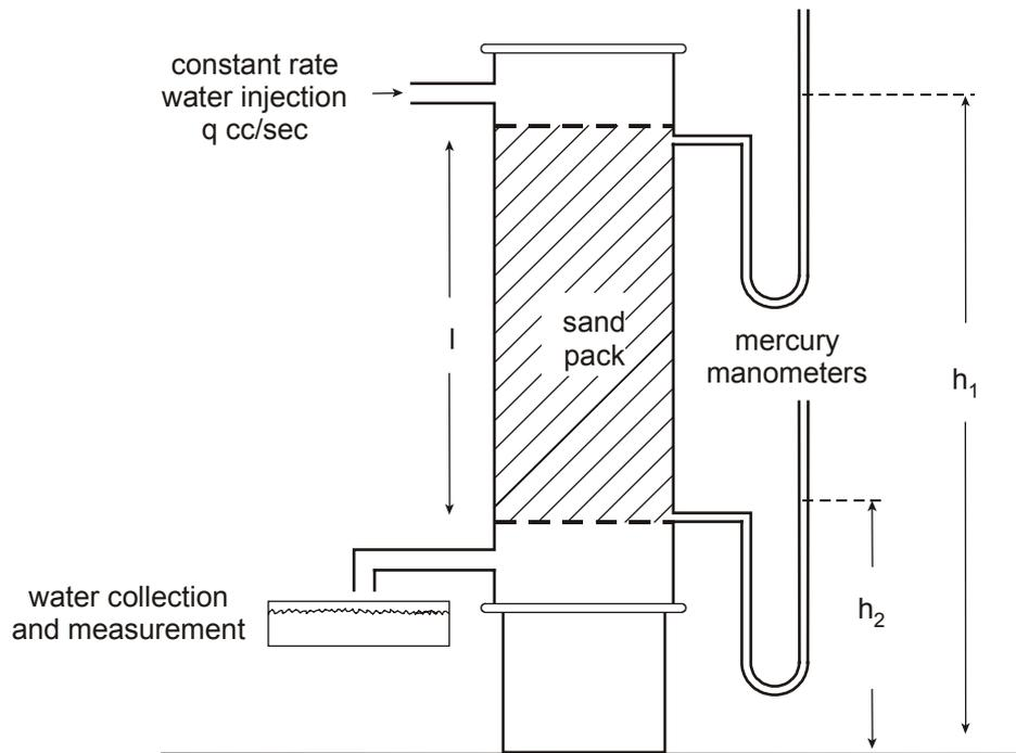
**Fig. 4.1 Schematic of Darcy's experimental equipment**
