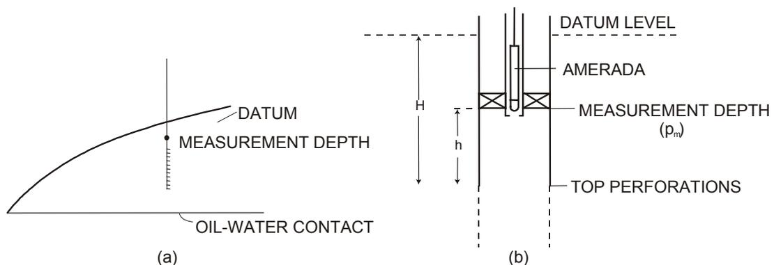
**Fig. 7.35 Correction of measured pressures to datum; (a) well position in the reservoir, (b) well completion design**
