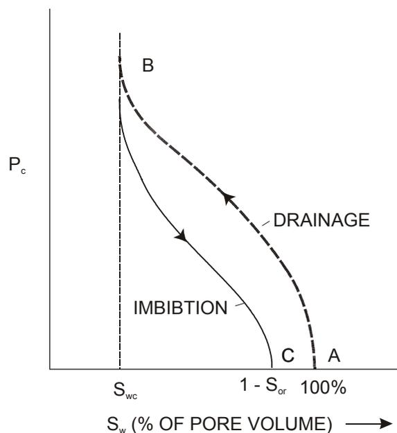
**Fig. 10.3** Drainage and imbibition capillary pressure functions
