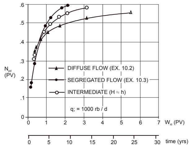
**Fig. 10.32** Comparison of oil recoveries for different assumed water saturation distributions during displacement.
