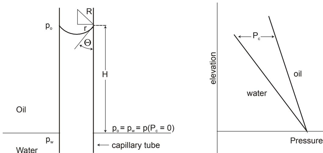
Fig. 10.4 Capillary tube experiment for an oil-water system
