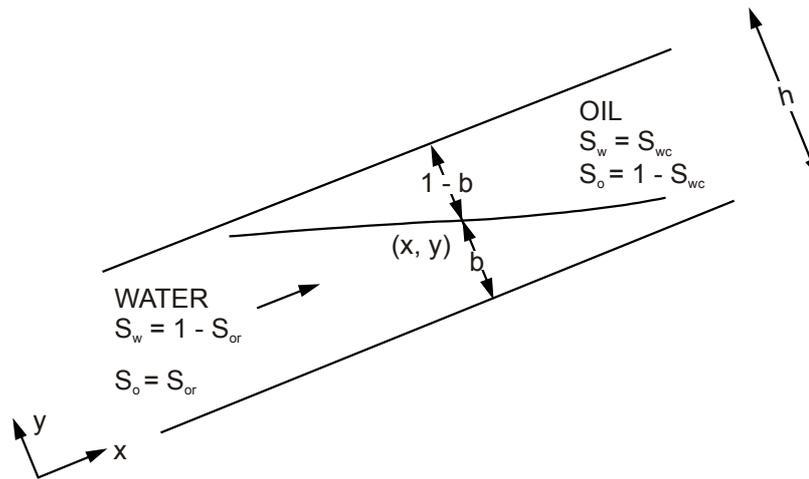
**Fig. 10.20 Segregated displacement of oil by water**
