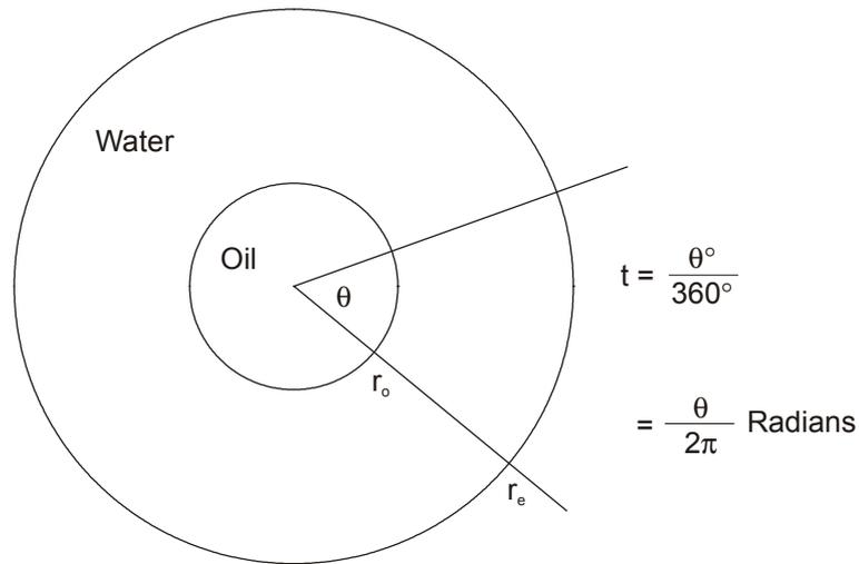
Fig. 9.1 Radial aquifer geometry
