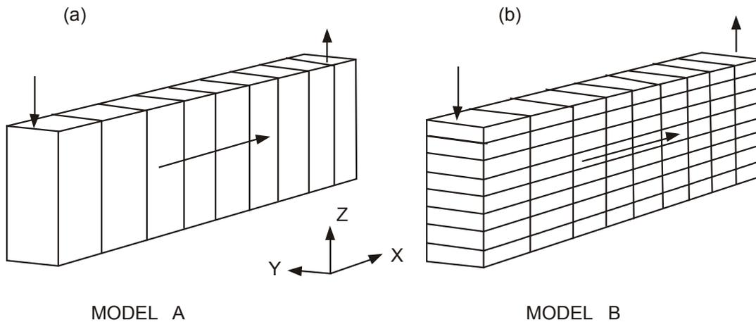
**Fig. 10.49 Alternative linear cross sectional models required to confirm the existence of vertical equilibrium**
