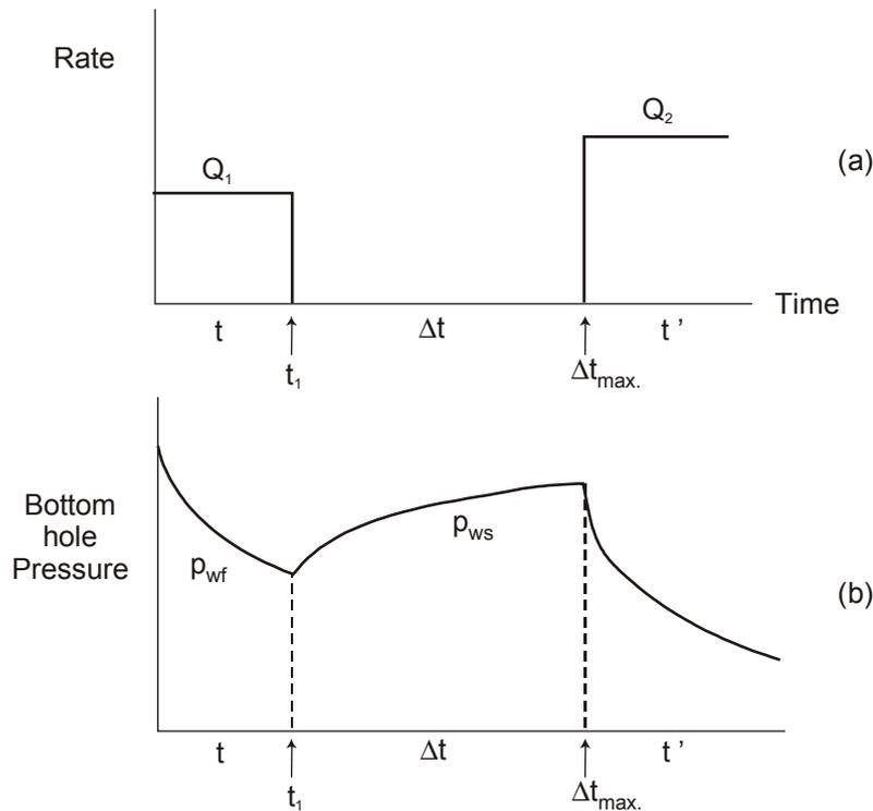
**Fig. 8.14 (a) Rate-time schedule, and (b) corresponding wellbore pressure response during a pressure buildup test in a gas well**
