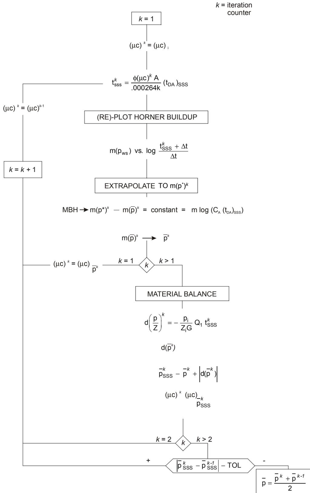
Fig. 8.17 Iterative determination of  $\bar{p}$  in a gas well test analysis (Kazemi<sup>10</sup>)
