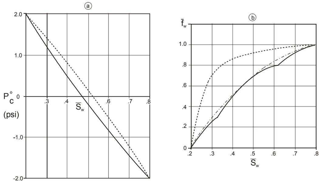
**Fig. 10.42 (a) Pseudo capillary pressures, and (b) fractional flow curves, exercise 10.4**
