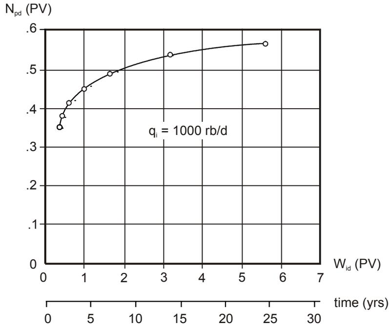
**Fig. 10.17 Dimensionless oil recovery (PV) as a function of dimensionless water injected (PV), and time (exercise 10.2)**
