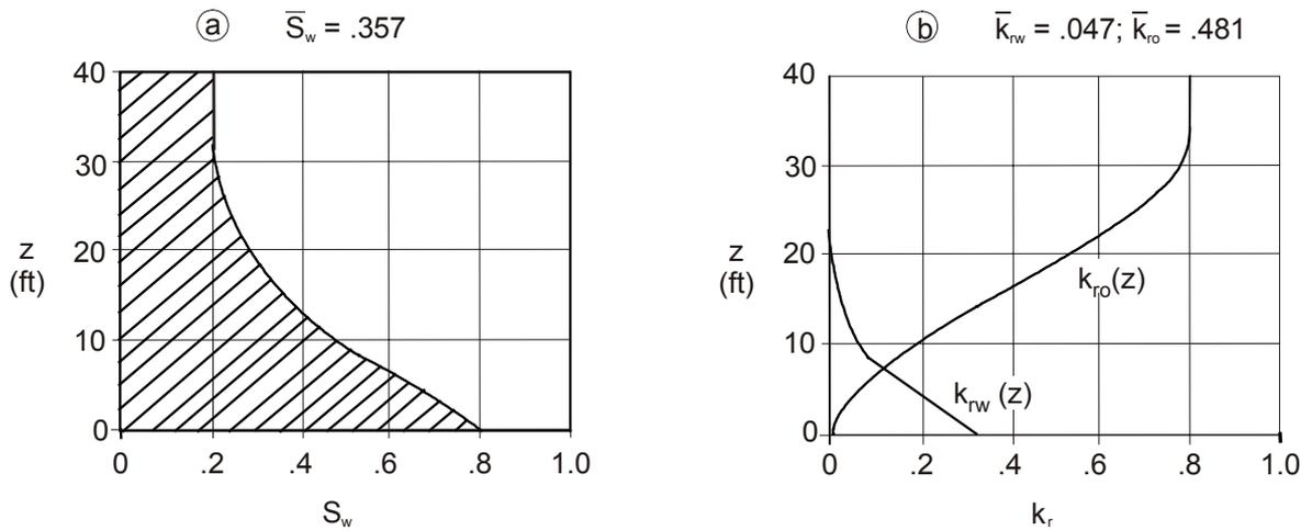
**Fig. 10.28 (a) Water saturation, and (b) relative permeability distributions, with respect to thickness when the saturation at the base of the reservoir is  $S_w = 1 - S_{or}$  ( $P_c = 0$ )**
