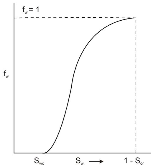
**Fig. 10.9** Typical fractional flow curve as a function of water saturation, equ. (10.12)
