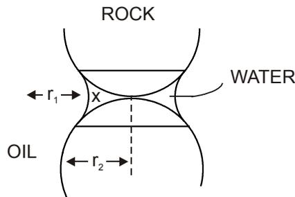
**Fig. 10.2** Water entrapment between two spherical sand grains in a water wet reservoir
