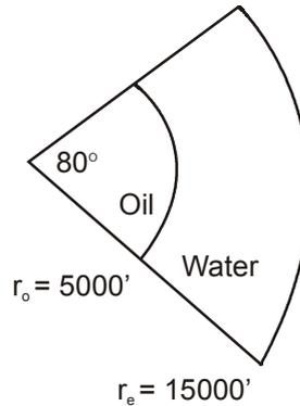
**Fig. 9.8 Water influx from a segment of a radial aquifer**
