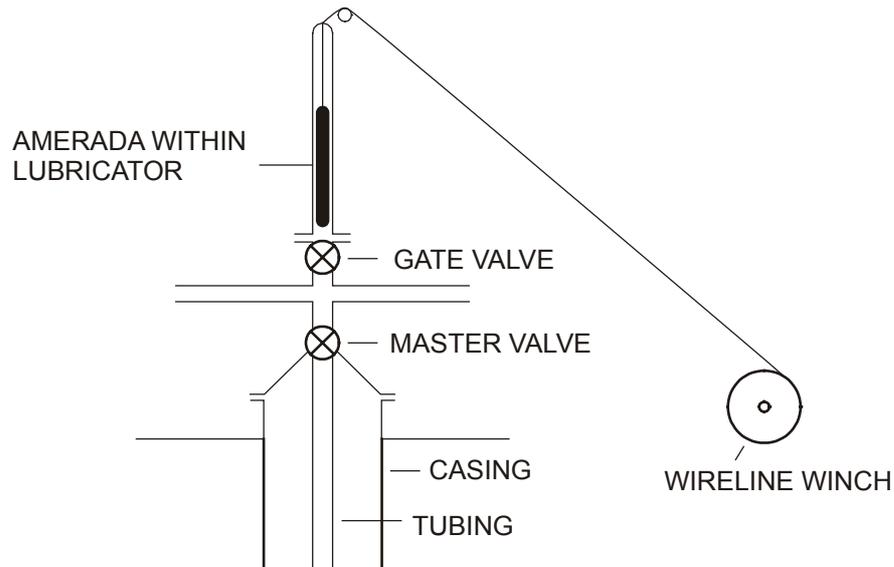
**Fig. 7.34 Lowering the Amerada into the hole against the flowing well stream**
