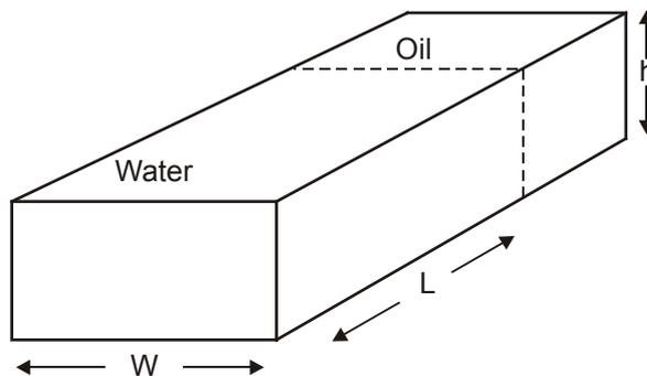
Fig. 9.2 Linear aquifer geometry
