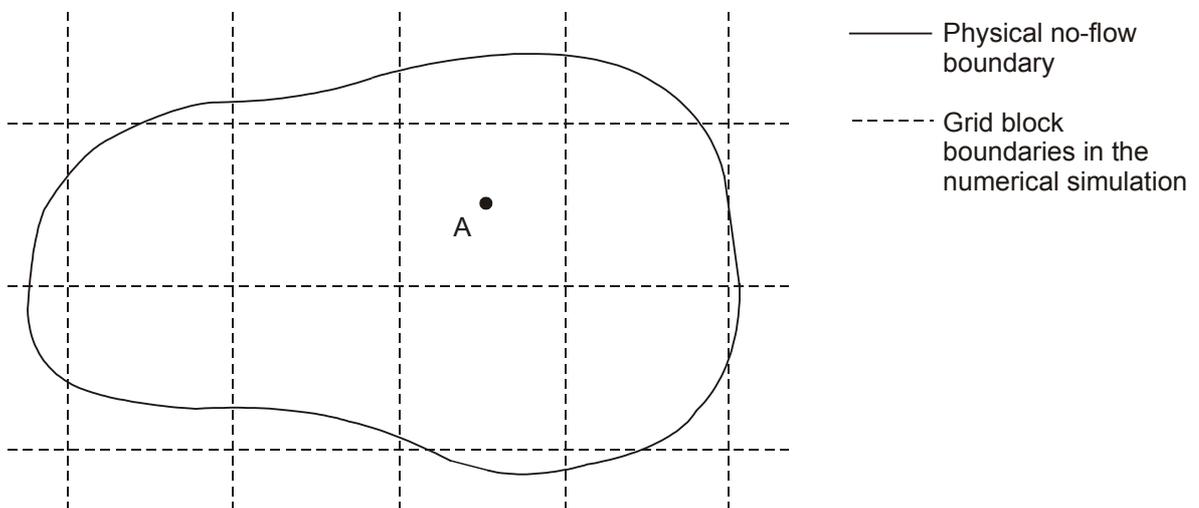
**Fig. 7.22 Numerical simulation model showing the physical no-flow boundary drained by well A and the superimposed square grid blocks used in the simulation**
