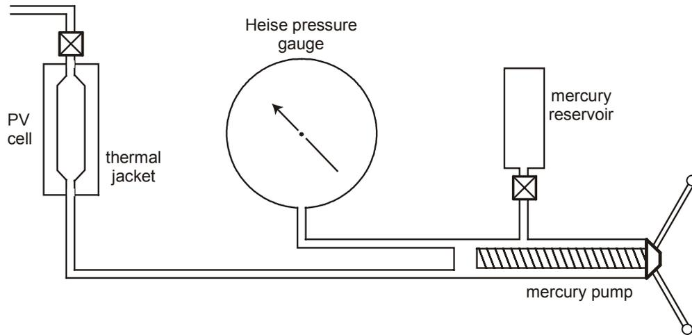
**Fig. 2.8 Schematic of PV cell and associated equipment**
