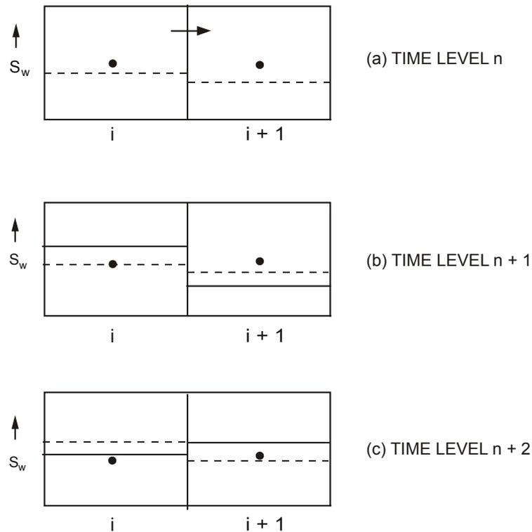
**Fig. 10.46 Example of water saturation instability (oscillation) resulting from the application of the IMPES solution technique (--- correct, and — incorrect saturations)**
