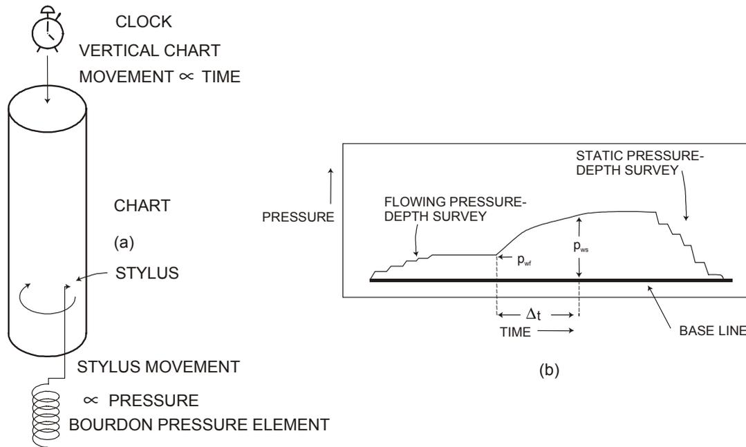
**Fig. 7.33 (a) Amerada pressure gauge; (b) Amerada chart for a typical pressure buildup survey in a producing well**
