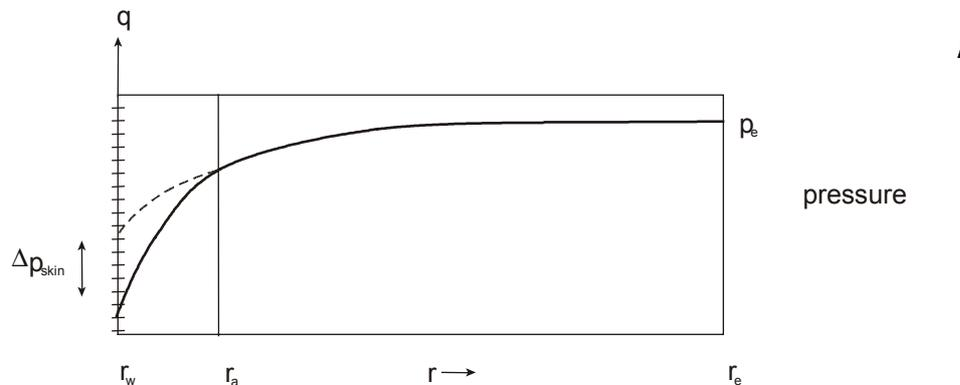
**Fig. 4.5 Radial pressure profile for a damaged well**
