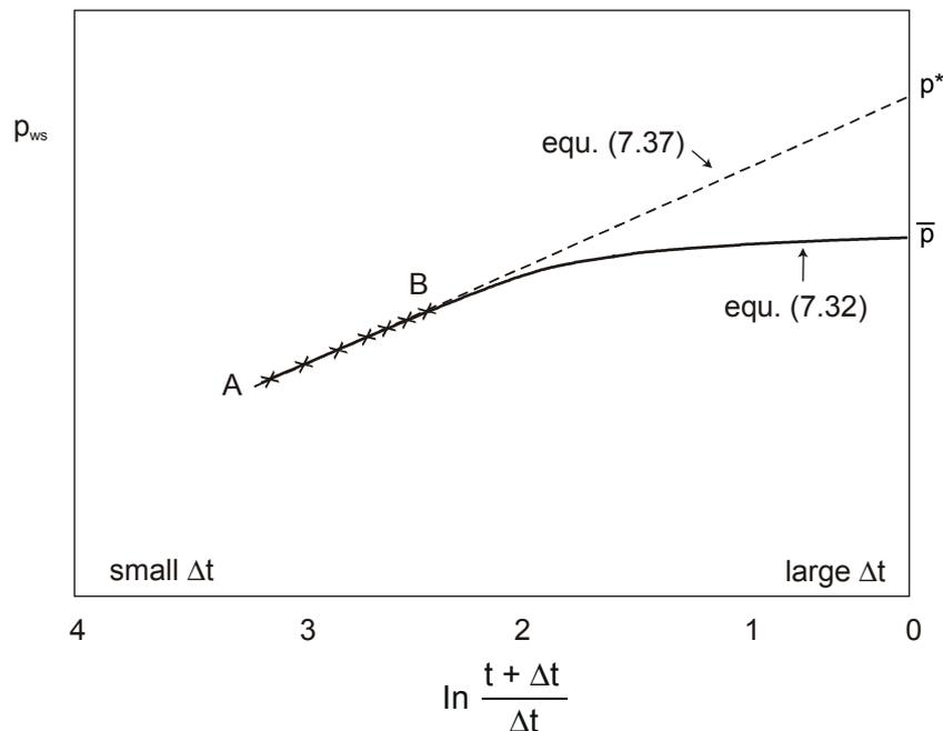
**Fig. 7.9 Horner pressure buildup plot for a well draining a bounded reservoir, or part of a reservoir surrounded by a no-flow boundary**
