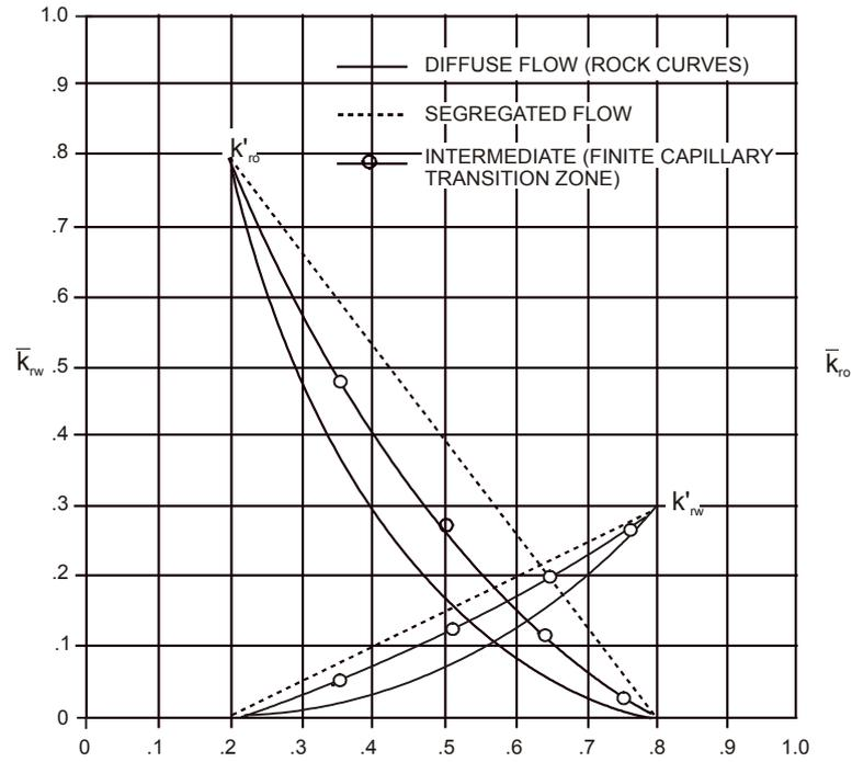
**Fig. 10.30** Averaged relative permeability curves for a homogeneous reservoir, for diffuse and segregated flow; together with the intermediate case when the capillary transition zone is comparable to the reservoir thickness
