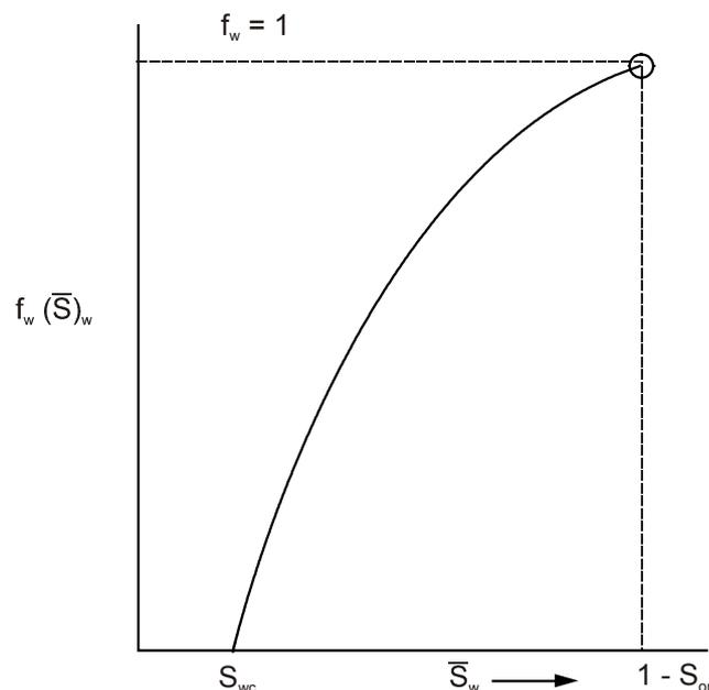
**Fig. 10.22 Typical fractional flow curve for oil displacement under segregated conditions**
