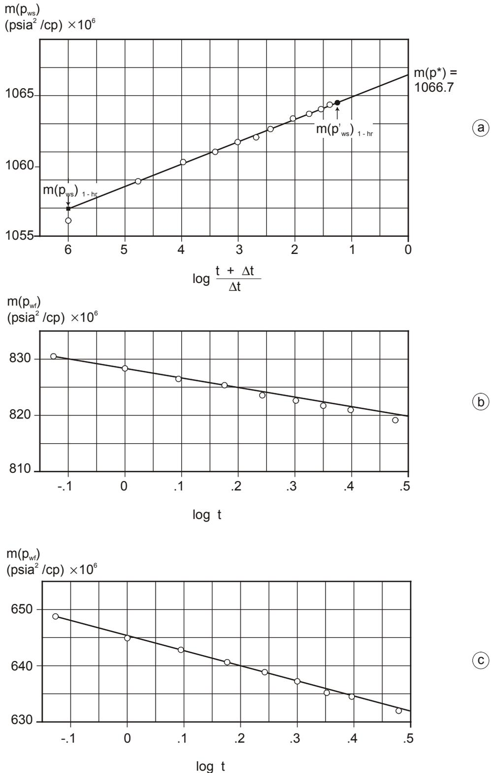
**Fig. 8.15** Complete analysis of a pressure buildup test in a gas well: (a) buildup analysis (table 8.12); (b) and (c) transient flow analyses of the first and second flow periods, respectively (table 8.10)
