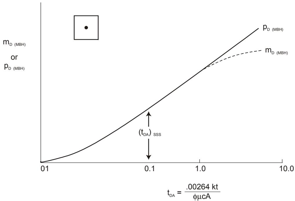
**Fig. 8.16 MBH plot for a well at the centre of a square, showing the deviation of  $m_{D(MBH)}$  from  $p_{D(MBH)}$  for large values of the dimensionless flowing time  $t_{DA}$**
