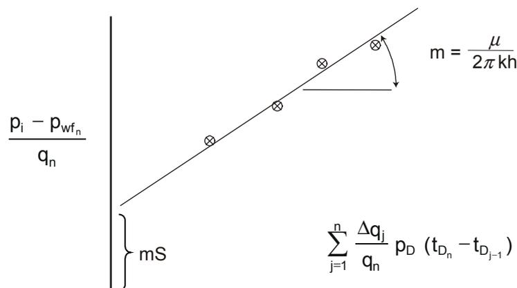
**Fig. 7.8 Multi-rate flow test analysis**
