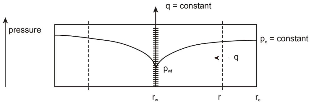
**Fig. 4.4 The radial flow of oil into a well under steady state flow conditions**
