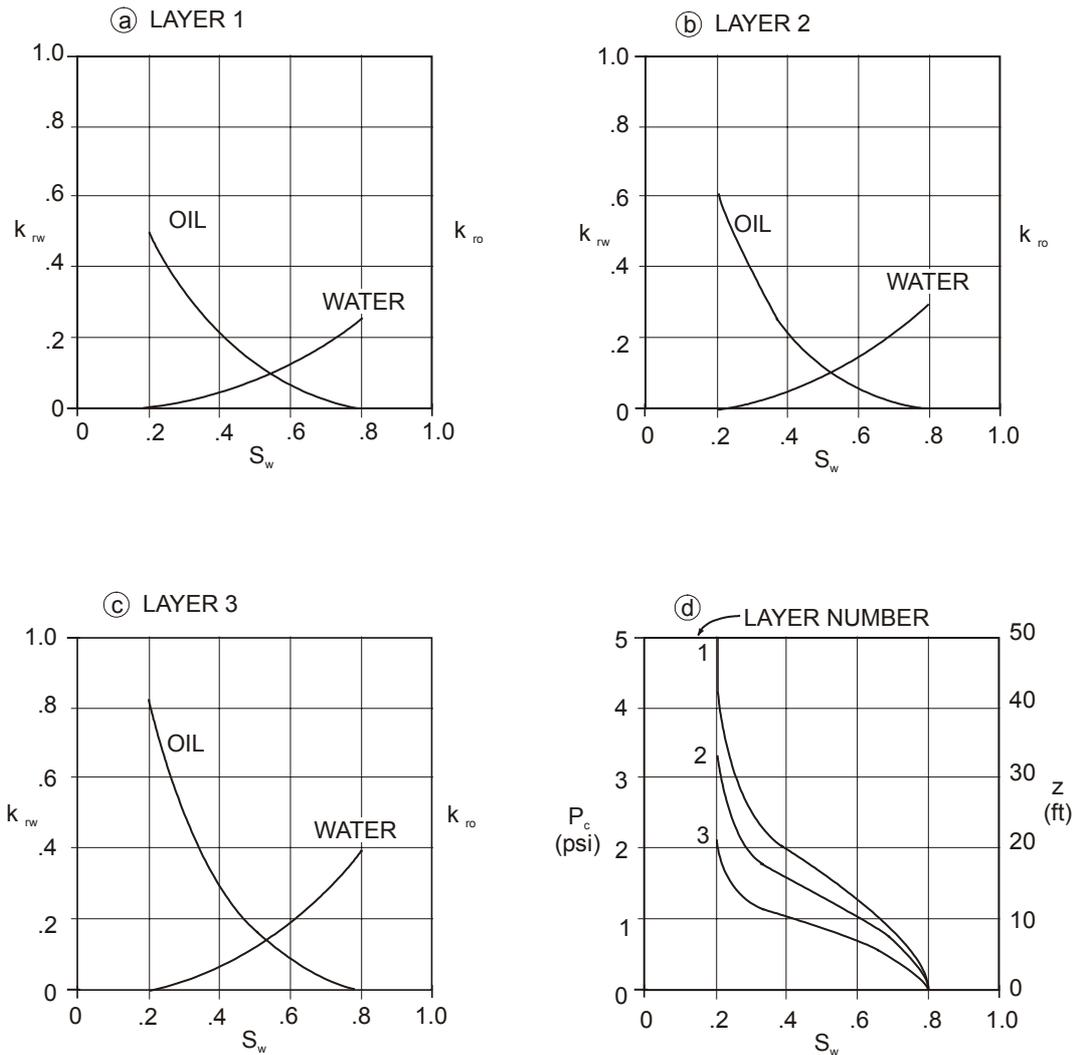
**Fig. 10.35 (a)-(c) Rock relative permeabilities, and (d) laboratory measured capillary pressures for the three layered reservoir shown in fig. 10.34**
