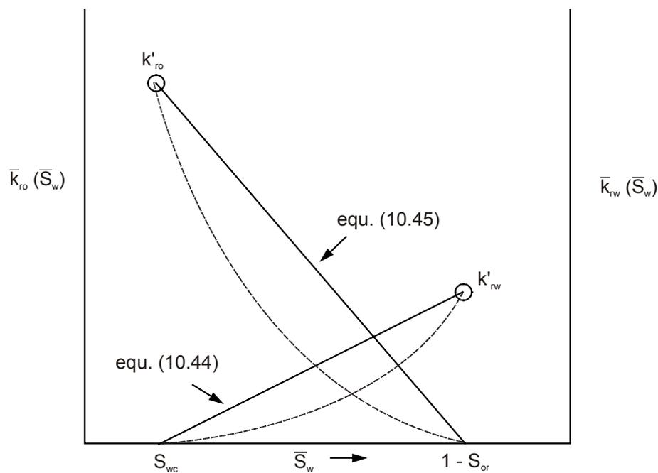
**Fig. 10.21 Linear, averaged relative permeability functions for describing segregated flow in a homogeneous reservoir**
