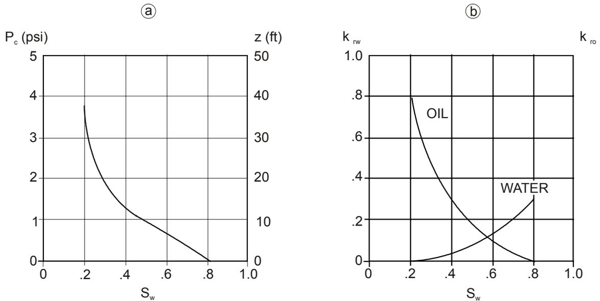
**Fig. 10.27 (a) Imbibition capillary pressure curve, and (b) laboratory measured relative permeabilities (rock curves, - table 10.1)**
