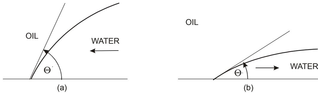
**Fig. 10.1 Hysteresis in contact angle in a water wet reservoir, (a) wetting phase increasing (imbibition); (b) wetting phase decreasing (drainage)**
