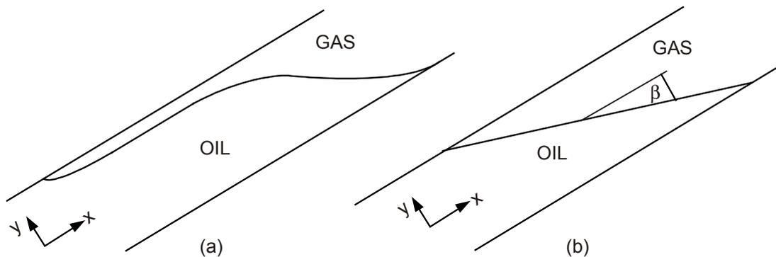
**Fig. 10.26 Segregated downdip displacement of oil by gas at constant pressure; (a) unstable, (b) stable**
