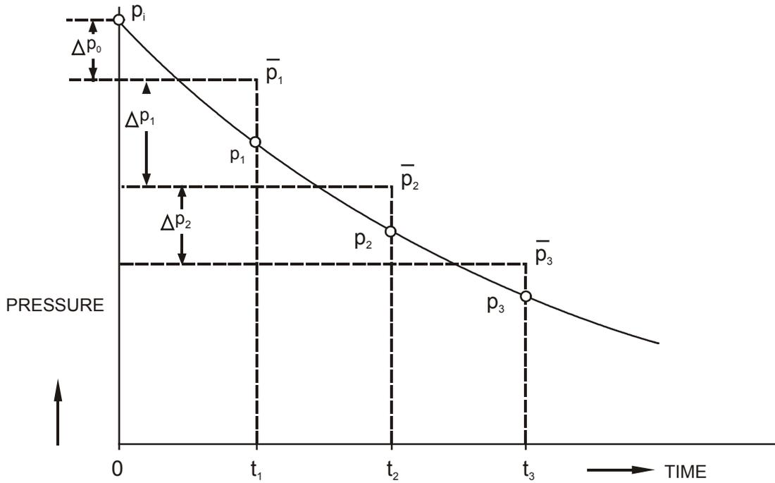
**Fig. 9.9** Matching a continuous pressure decline at the reservoir-aquifer boundary by a series of discrete pressure steps
