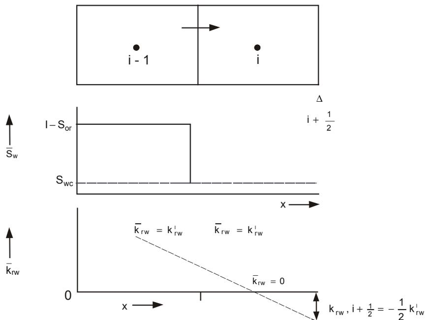
Fig. 10.48 Overshoot in relative permeability during piston-like displacement
