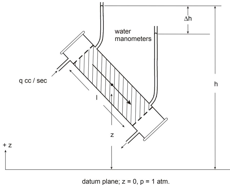
**Fig. 4.2 Orientation of Darcy's apparatus with respect to the Earth's gravitational field**
