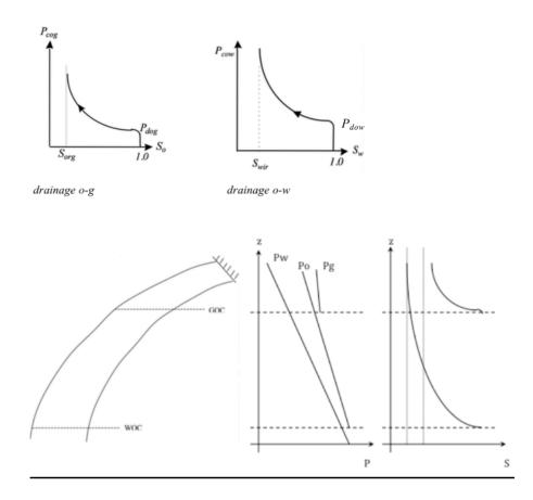
At the WOC Po-Pw=Pdow, and at GOC Pg-Po. Initial pressures are computed using densities and assuming equilibrium. At WOC Sw=1,0. At any z value, Pcow is computed from the difference in Po and Pw, and the corresponding Sw is found from the Pcow-curve. At GOC Sg=0. At any z-value above the corresponding Sg is found from the Pcog-curve
