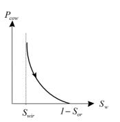
• A typical imbibition curve for a system that is partly oil wet.
