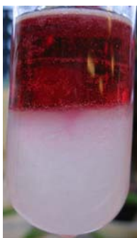
Figure 7: Dyed water on top of the plug shows that it is visibly impermeable. The presence of colour in the middle is where the nucleation promoting surface was removed. It can be seen that the colour does not penetrate the plug elsewhere. This test has been performed several times with the same results.
