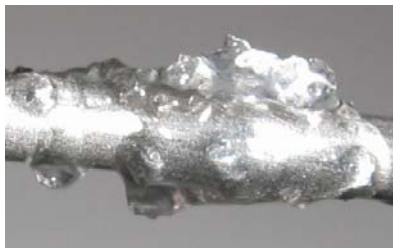
Figure 8: Hydrate crystals on the sensor of the thermometer
