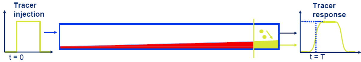
Figure 12 Tracer Response in Multiphase pipeline (Bjørnar 2005)
