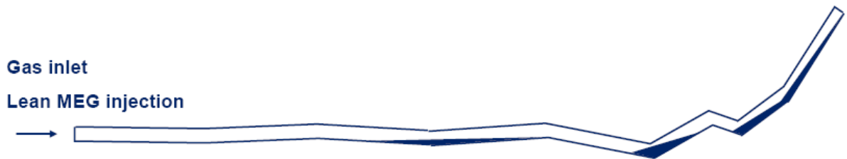
Figure 13 Pipeline with an undulating path (Bjørnar 2005)
