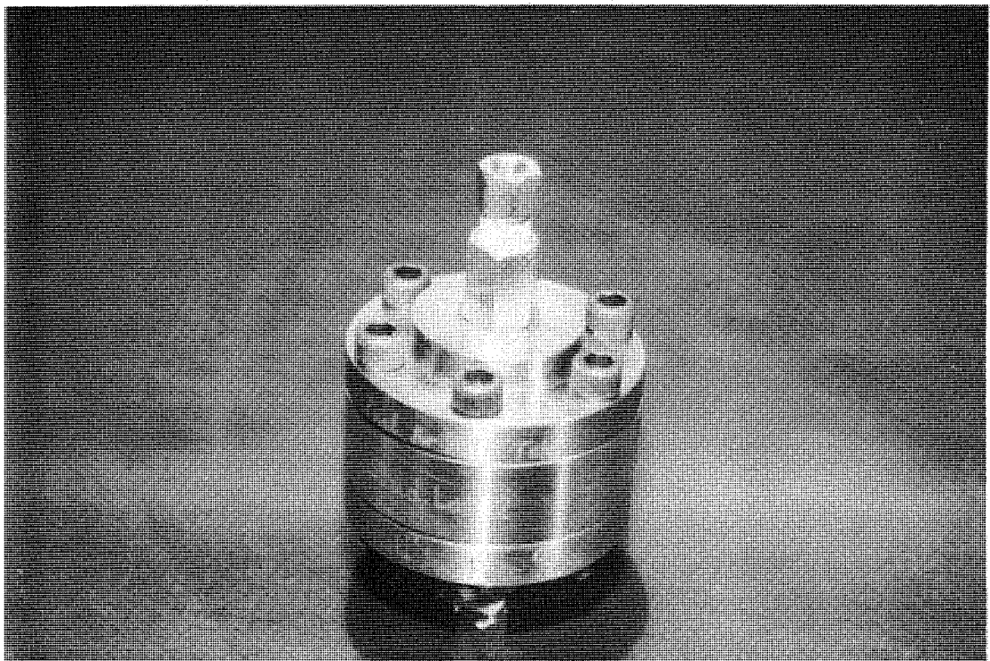
Fig. 3.28 Assembled high-pressure capillary pressure core holder
