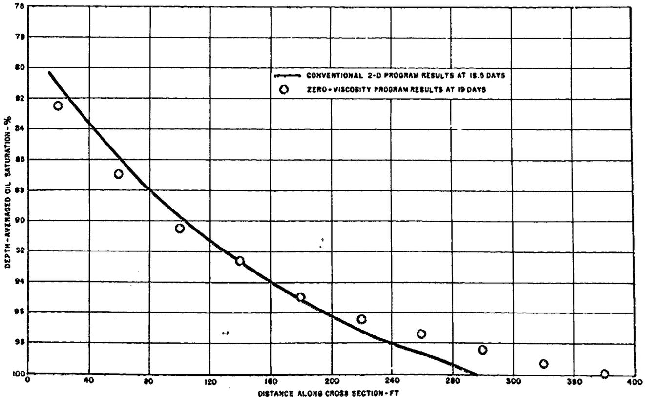
FIG. 4 — COMPARISON OF CONVENTIONAL TWO-DIMENSIONAL AND ZERO VISCOSITY PROGRAM RESULTS AT 18.5 PERCENT OF CRITICAL RATE.
