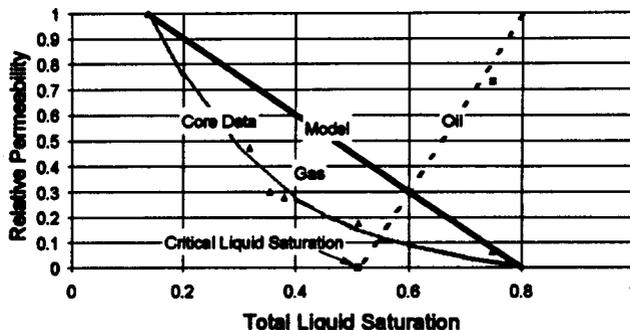
Figure 9 - Model gas relative permeability curve
