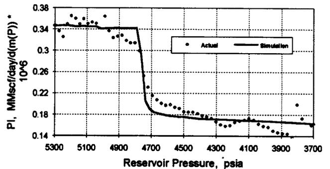
Figure 19 - PI of the 6-layer model vs. the actual Arun well
