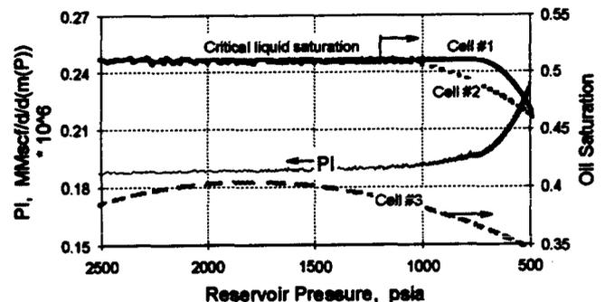
Figure 15 - Effect of liquid revaporization on PI
