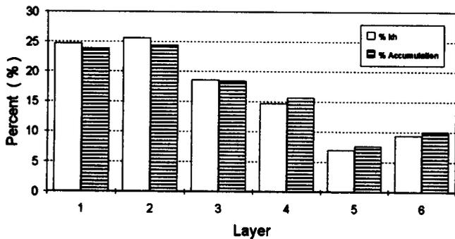
Figure 17 - Condensate accumulation in different layers
