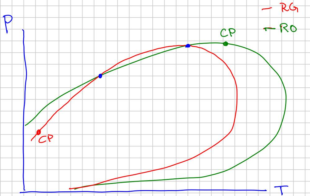
• Saturated Gas-Oil System (<sup>Gas Cap +</sup><sub>Oil Zone</sub>)
