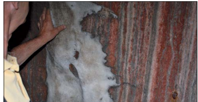
Figure 4 Thin clay layers (dark grey) embedded in the halite (white and red).
