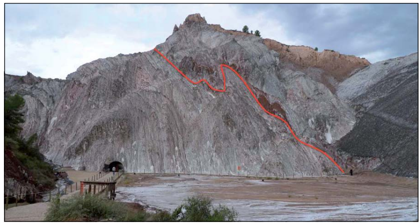
Figure 13 Trace of the shear zone (red line) at outcrop, probably corresponding to the shear zone in the mine gallery (Figure 12).
