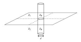
Figure 1: Parameters defining diffraction response from borehole: diameter d and impedance contrast of borehole  $(Z_B)$  with host rock  $(Z_1, Z_2)$ .
