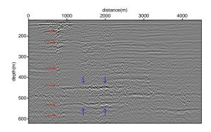
Figure 8: Time lapse diffraction image. Red arrows: relief well; blue arrows: anomaly due to gas blow out.
