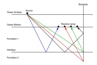
Figure 2: Responses in borehole model: reflection (blue), diffraction on borehole head (red), diffraction on borehole-interface intersection (green), prismatic reflection (black).
