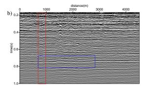
Figure 4: LOSEM data raw stack. a) 1988, b) 1990. Red box: seismic response from relief well; blue box: anomaly due to gas blow out.
