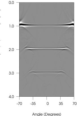
Figure 4: Angle gather computed using Rickett and Savas(2002) offset imaging condition by employing equation 11 and then using equation 10.
