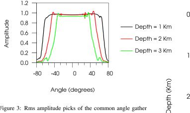
Figure 3: Rms amplitude picks of the common angle gather shown in Figure 2(b)
