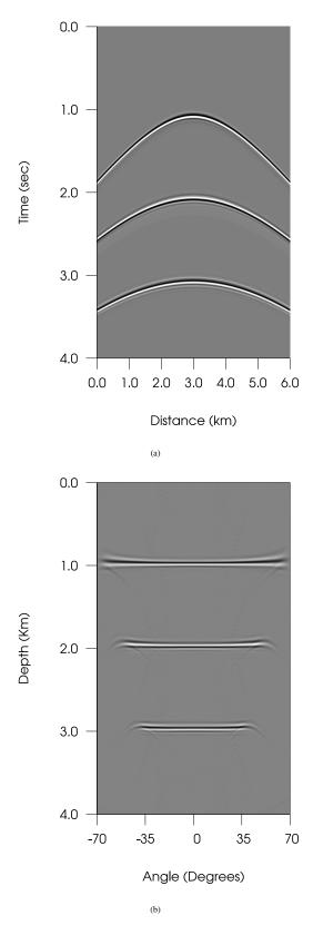
Figure 2: Single shot (a) acquired over the earth model shown in figure 1 The acquisition geometry is of split-spread type with maximum half offset of 5 km. A common angle gather (b) was computed using equation 10 and 200 shots.
