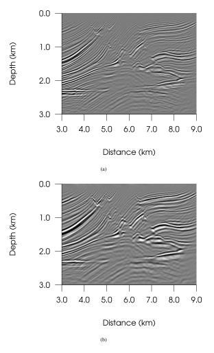
Figure 6: (a) Zero-offset section using the Marmousi synthetic data set with the true-amplitude imaging condition given by equation 9 and (b) zero-offset section using the Marmousi synthetic data set and the Claerbout cross-correlation imaging condition.
