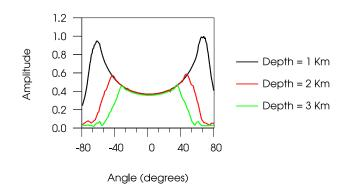
Figure 5: Rms amplitude picks of the common angle gather shown in Figure 4.
