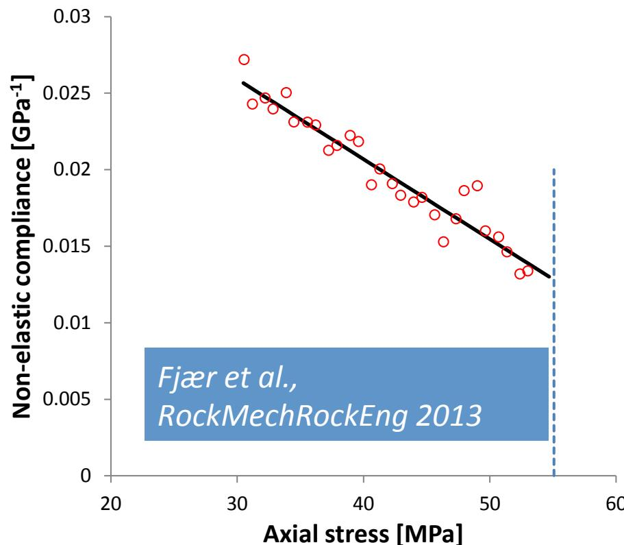
The non-elastic compliance should disappear near turning points of the stress path, where the material behaves elastically
