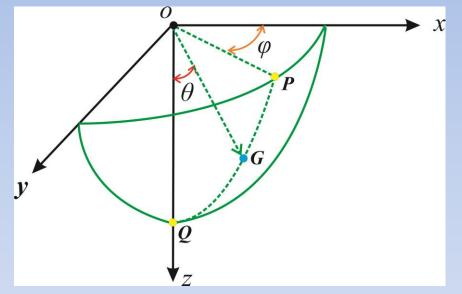
Figure 2: Schematic plot for the anelliptic approximation of P-wave phase velocity. G is a point on the P-wave phase velocity surface (formed by green solid lines).
