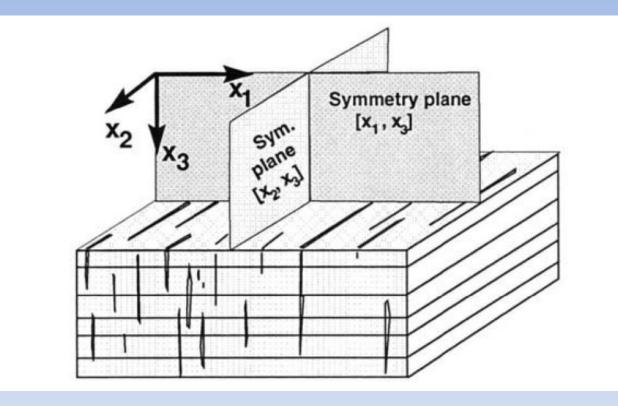
Figure 1: Orthorhombic model caused by parallel vertical fractures embedded in a finely layered medium.(Tsvankin, 2001). In this presentation,  $x_1$ -,  $x_2$ - and  $x_3$ -axes correspond to x-, y-, z-axes, respectively.
