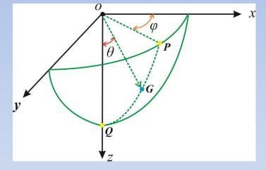
Figure 2: Schematic plot for the anelliptic approximation of P-wave phase velocity.
