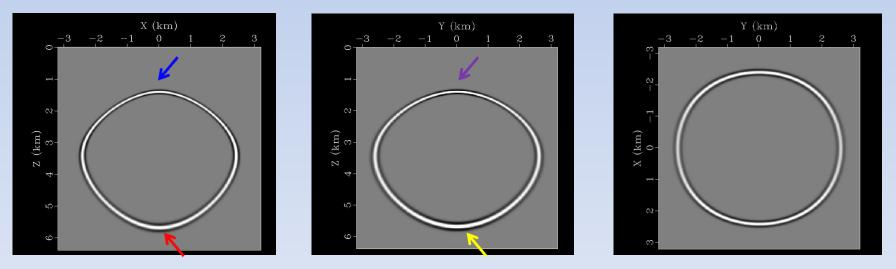
Figure 9: Three slices for the wavefield snapshot at t=0.8s in a 3D vertically factorized orthorhombic medium. All slices cross the position of source.
