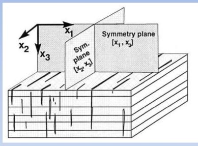
Figure 1: Orthorhombic model caused by parallel vertical fractures embedded in a finely layer medium.(Tsvankin, 2001). In this presentation, x1-, x2- and x3-axes corresponds to x-, y-, z-axex, respectively.
