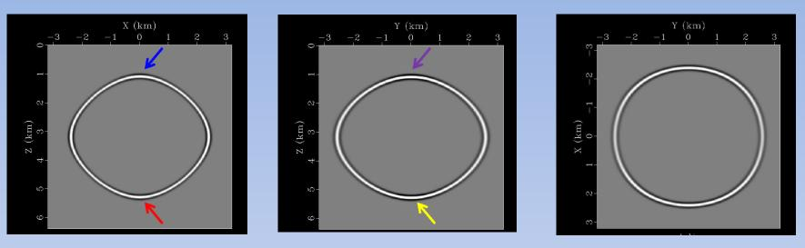
Figure 8: Three slices for the wavefield snapshot at t=0.8s in a 3D homogneous orthorhombic medium. All slices cross the position of source.
