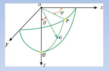
Figure 2: Schematic plot for the anelliptic approximation of P-wave phase velocity.
