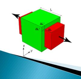
Poisson's ratio, v: ratio of transverse contraction to axial extension
