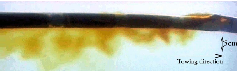
Above: seismic streamer is cross-flow
