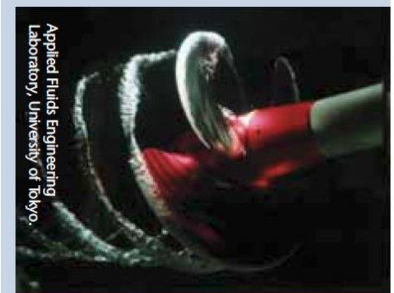
Picture of bubble (top) and propeller cavitation.
