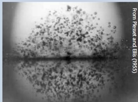
Photograph of a transient cloud of cavitation bubbles generated acoustically.
