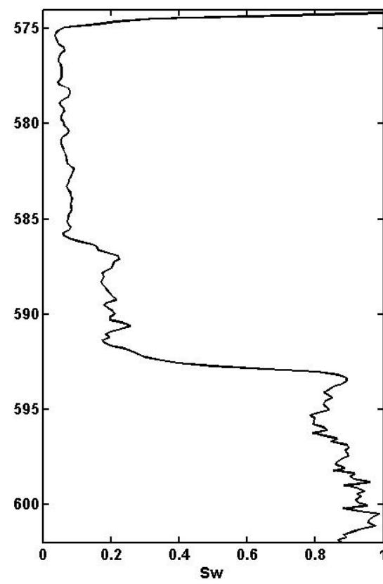
Detail showing that the saturation increase at 592 m correlates with a density increase of 0.12 g/ccm
