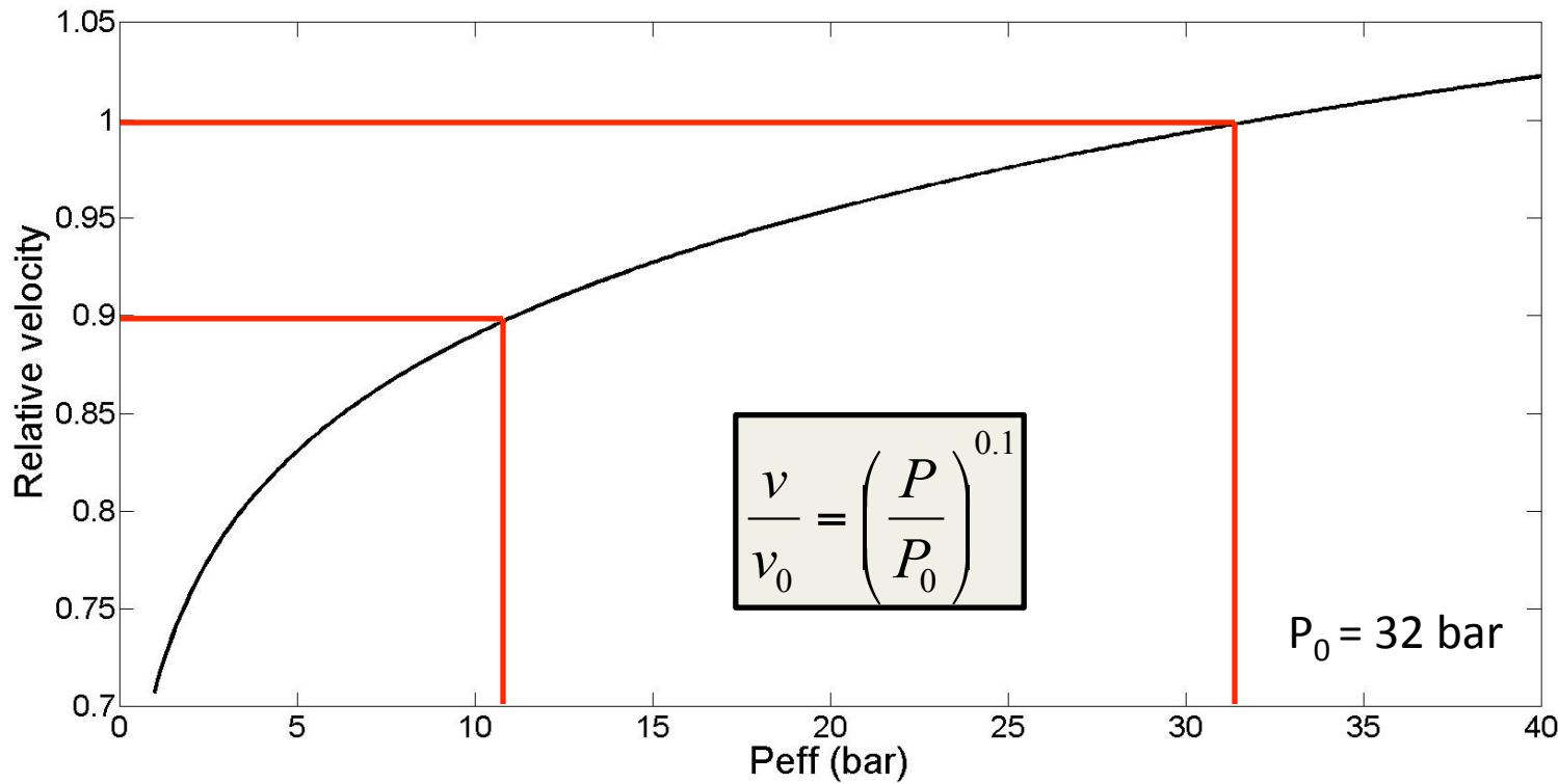
A reduction in effective pressure of 21 bar => 10 % reduction in P-wave velocity
