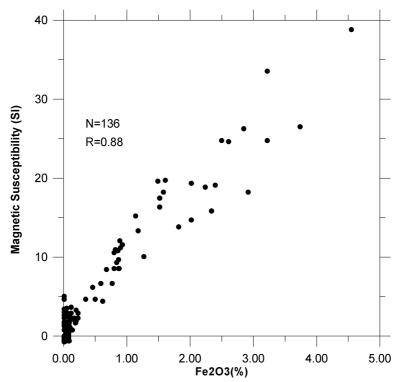
Figure 5. Magnetic susceptibility versus Fe<sub>2</sub>O<sub>3</sub>.
