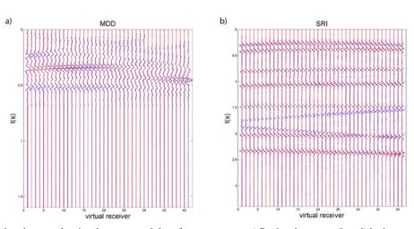
Figure 3: Comparison between the virtual response and the reference response. a) Retrieved response (in red) by inter-source SI using MDD compared with the reference response (in blue) modelled with a homogeneous overburden. b) Retrieved response (in red) by SRI compared with the reference response (in blue) modelled with a homogeneous underburden. The direct waves are removed in both panels.
