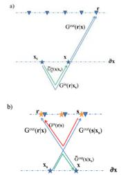
Figure 1: Illustration of the survey geometries. a) The acquisition geometry for the inter-source SI by MDD scheme. b) The acquisition geometry for the SRI scheme. The stars denote sources and the triangles denote receivers. The color green indicates the propagation path for the retrieved virtual response.
