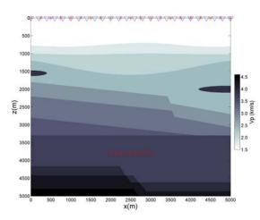
Figure 2: Geometry of the numerical experiment with the velocity model used. The blue triangles denote receivers and the red stars denote sources.
