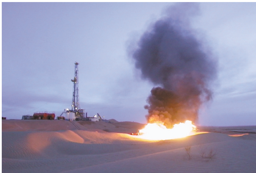
Figure 1. Flow testing a well is always an awe-inspiring event. Adding to the enjoyment, Annaeem 1 flowed hydrocarbons from porous, permeable sands in an area where Alif sands were long thought not present.
