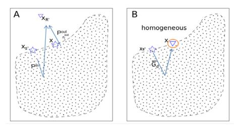
Figure 1 Configurations of state A and B for inter-source SI by MDD. The dotted line describes the boundary enclosing the integral volume. The orange circle denotes the virtual receiver. The star denotes a source and the triangle denotes a receiver.
