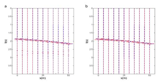
*Figure 4* Comparison of the retrieved response and the reference response. a) Retrieved response by *CC* (*red*) compared with the reference response (blue). Every fifth trace is plotted. b) Retrieved response by *MDD* (*red*) compared with the reference response (blue).
