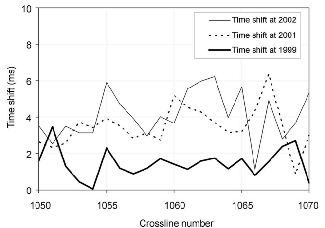
Figure 14. Estimated time shift caused by the CO 2 side-plume event, measured on the base of the Utsira Sand.
