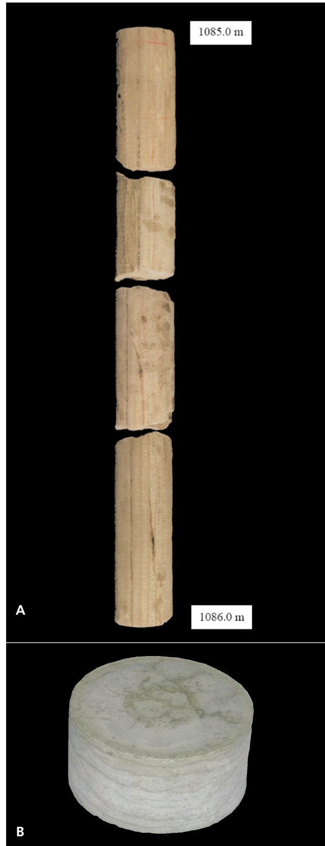
Figure 3 Photos of core material from Sleipner: (a) Utsira Sand and (b) cap rock.
