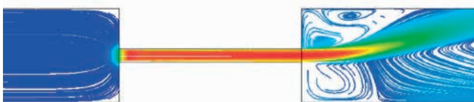
2D streamlines depicting velocity magnitude of fluid passing through a bean choke
