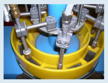
Wet High Intensity Magnetic Separation (WHIMS). Close-up of the matrix boxes of the Jones P40 pilot scale separator. Photo: Oppredningslaboratoriet.
