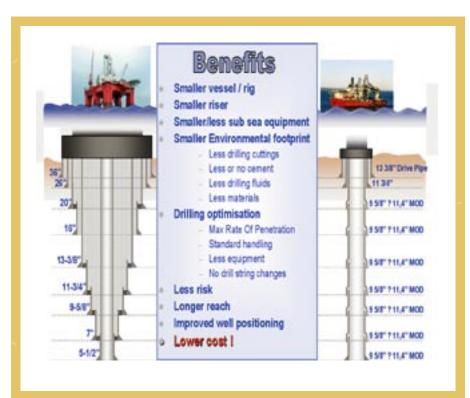
Illustration of step-change in technology by implementing Monodiameter technology. (ex. 9 5/8" expanded to 11.4")
