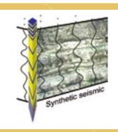
The SOP project – comprises multidisciplinary collaboration between geology and seismics on resolving reservoir heterogeneity by modeling seismic signals from real geological data, through upscaling petrophysical properties using SBED.
