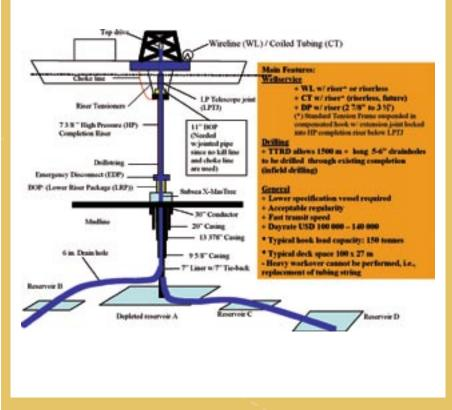
Set-up for Effective Well Intervention and Drain Hole Drilling using Through Tubing Rotary Drilling (TTRD)
