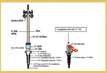
Figure 4.5 Low Cost Drilling and Completion Concept (11" wellhead)
