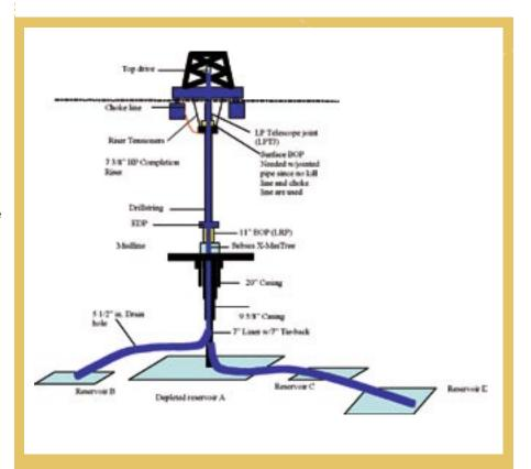
Figure 4.4 Set-up for TTRD
