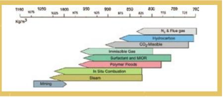
Figure 5.1 Most effective oil density range for various EOR methods.
