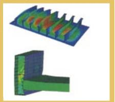
Simulation of stiffened plate response and ice floe-tanker side interaction
