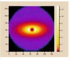
Asymmetric pores parallel to layers
