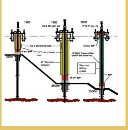
Figure 5.5 Trends in deepwater drilling technology
