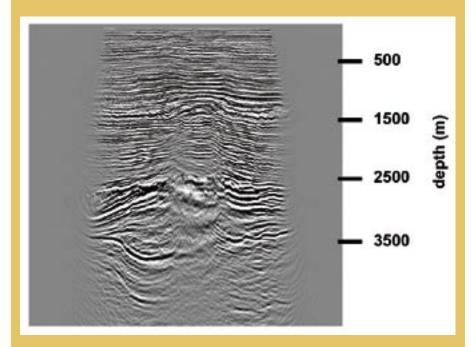
Figure 5.18 The same line as in Fig. 5.17, but extracted from a 3D wavefield (common receiver) migration.
