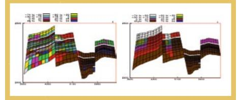
Figure 5.13: Estimated (left) and real (right) pore pressure changes for a synthetic example based on a North Sea field reservoir model (from Mohsen Dadahspor's Ph.D. work).
