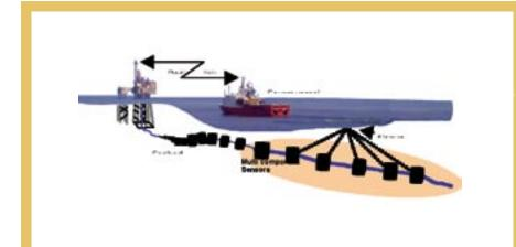
Figure 7.2 Ocean Bed Seismic data acquisition with a permanently installed cable.
