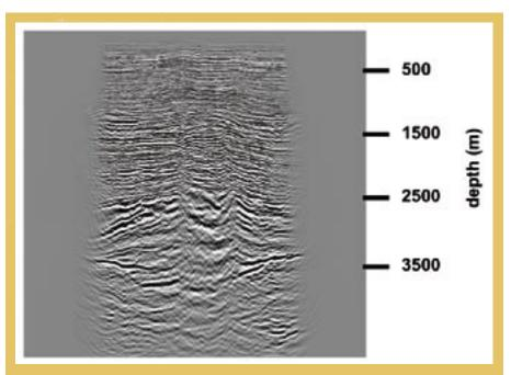
Figure 5.17 P-wave angle migration result through the gas cloud at the Valhall Field.
