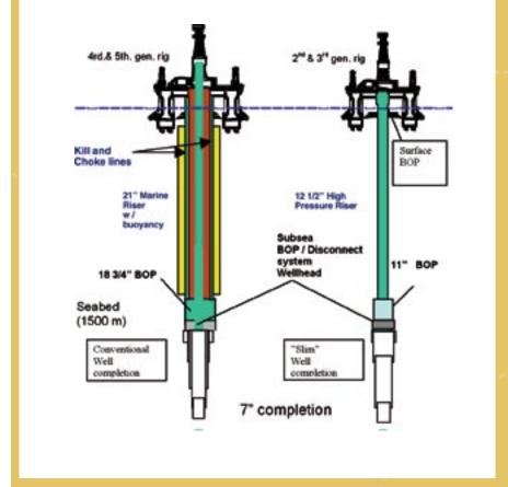
Figure 4.2 Conventional vs. potential "slim hole" drilling system
