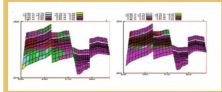
Figure 5.14: Estimated (left) and real (right) water saturation changes for a synthetic example based on a North Sea field reservoir model (from Mohsen Dadahspor's Ph.D. work).
