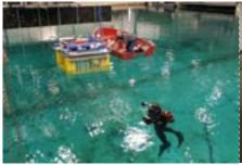
Testing of a floating production platform model including risers and anchor system in the Ocean Basin Laboratory.
