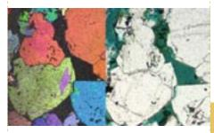
SEM EBSD techniques (left) can be used to map mineral orientation (right: optical micrograph).
